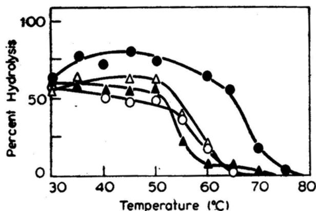
**Figure 2.** Heat denaturation of the four enzyme proteins. Enzymes were kept at required temperature for 10 min (in a water bath), chilled and immediately assayed for the four activities as given in the text.
