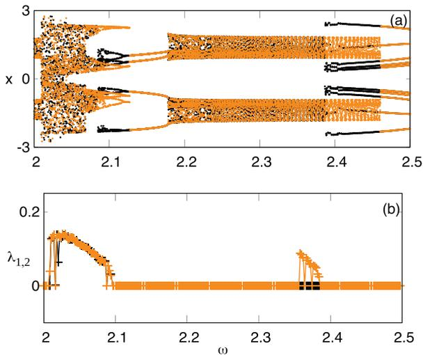
**Figure 1.** (a) Bifurcation diagram depicting the multistability of eq. (1) and (b) the two largest Lyapunov exponents of the system with respect to the generator’s frequency  $\omega$ . The parameters are fixed as  $\mu = 0.9$ ,  $\beta = 0.5$  and  $\epsilon = 0$ . The black and orange dots represent two different bifurcation scenarios of the model for the same set of parameters with initial conditions  $[x_0, y_0, z_0] = [2, 0, 0.7]^T$  and  $[-1, 0, 0.5]^T$  respectively.
