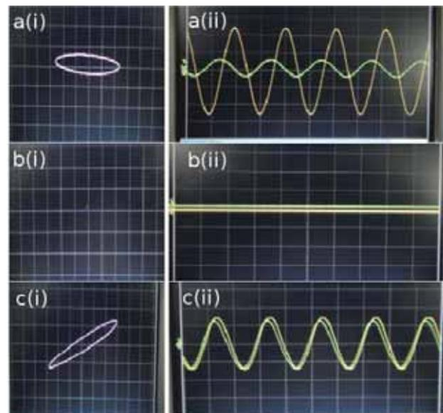
**Figure 3.** Experiment: (i) Phase space and (ii) time series of the three dynamical regimes: (a) anti-phase, (b) AD and (c) in-phase regimes.
