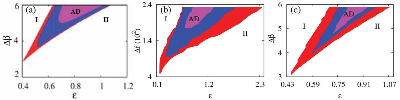
**Figure 2.** Phase diagrams of the coupled Chua's oscillators. (a) Numerical study in the  $(\epsilon - \Delta\beta)$  plane and (b) experimental observation in the  $(\epsilon - \Delta f)$  plane. (c) For the coupled fractional order Chua's circuit in the  $(\epsilon - \Delta\beta)$  plane as a function of order  $q_2$  of the system.
