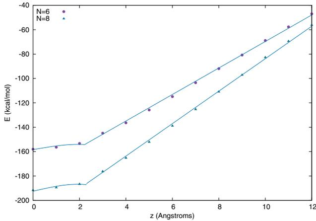
**Figure 1.** Plots of interaction energy  $\Delta E$  vs. axial distance  $z$  for  $N = 6$  and  $N = 8$  for 12 Å long DWCNTs. Data points are obtained from DFT calculations, while solid curves are obtained from the nonlinear spring model.
