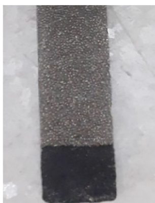
Figure 2. Active material coated on nickel foam.
