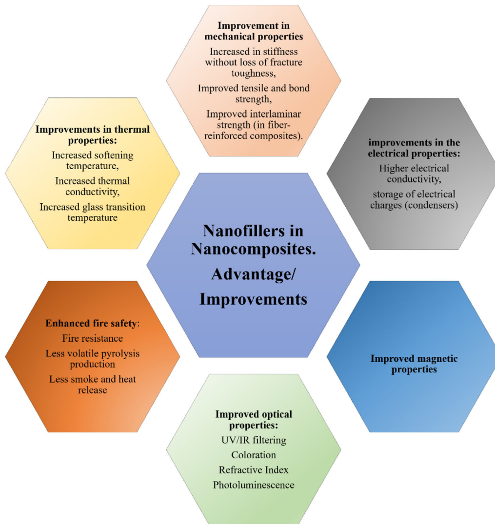
Figure 3. Improvements and advantages of the introduction of nanofiller into the nanocomposites.
