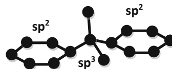
Figure 5. Schematic representation of crosslinked sp^2 and sp^3 carbon clusters, while the orientation mismatch presents geometrical hurdle for compressive forces though bending might be preferred.
