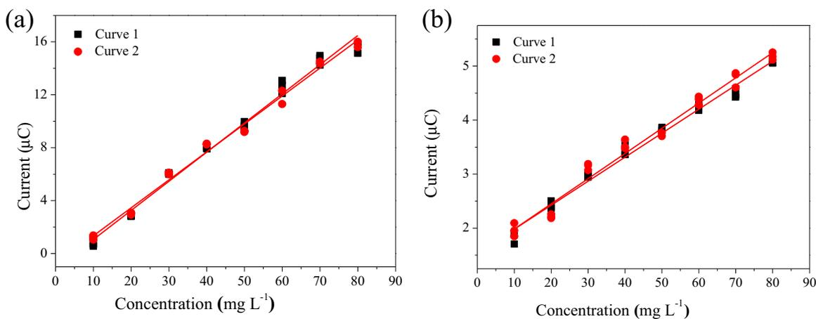
**Figure 10.** Precision study for the voltammetric method using analytical curves obtained with same analyst using different modified (a) GCE–EG and (b) GCE–CNT electrodes.
