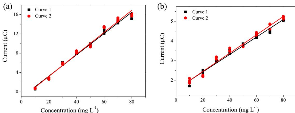
**Figure 9.** Precision study for the proposed voltammetric method using the analytical curves obtained with the same analyst using the same electrodes: (a) GCE–EG and (b) GCE–CNT.
