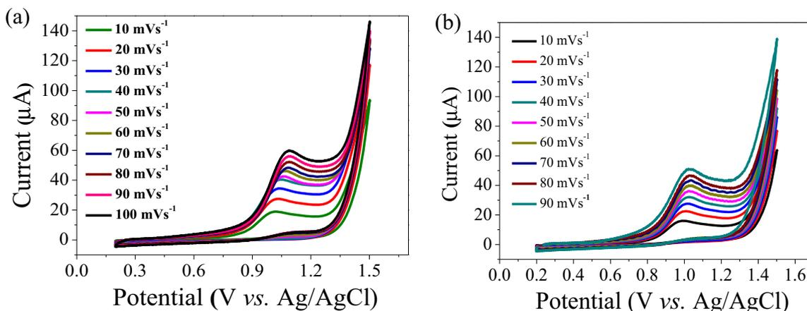
**Figure 6.** Cyclic voltammograms for 80 mg l<sup>-1</sup> of morpholine, in an electrolyte solution in 0.1 mol l<sup>-1</sup> of KCl (pH 10) varying the scan speed from 10 to 90 mV s<sup>-1</sup> using (a) GCE-EG and (b) GCE-CNT.
