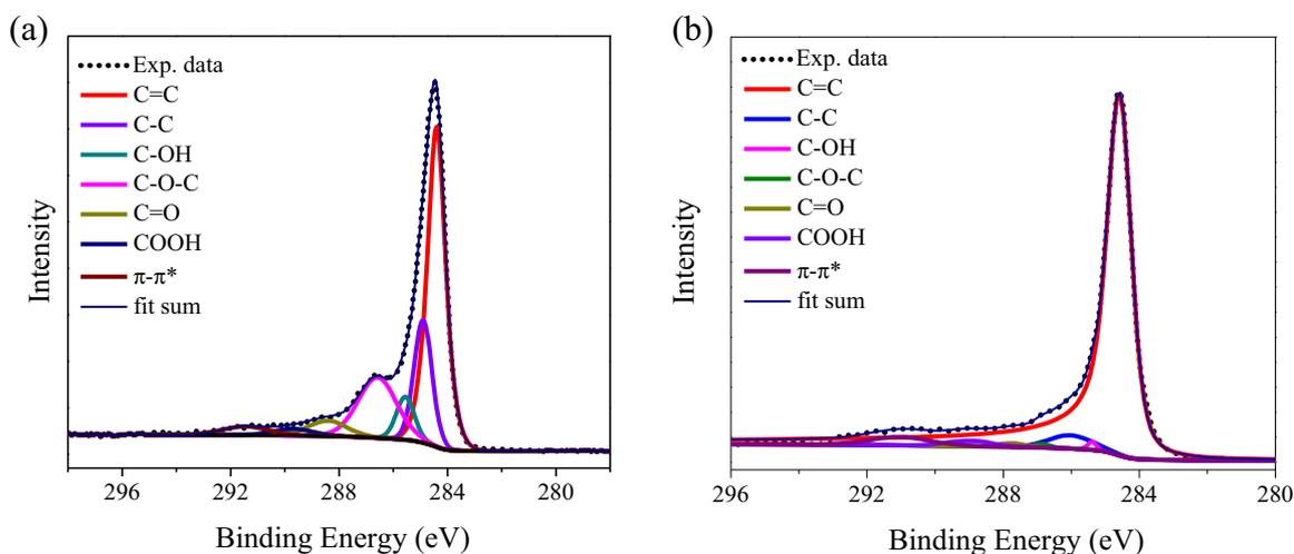
**Figure 4.** High-resolution C1s spectra of (a) EG and (b) CNT samples.
