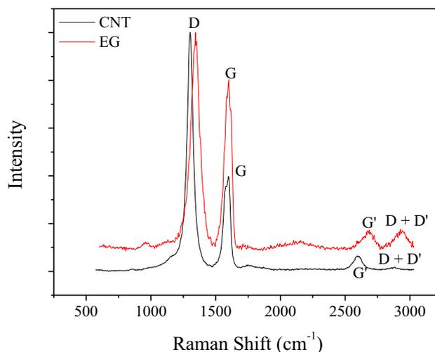
**Figure 2.** Raman spectra of EG and CNT samples.
