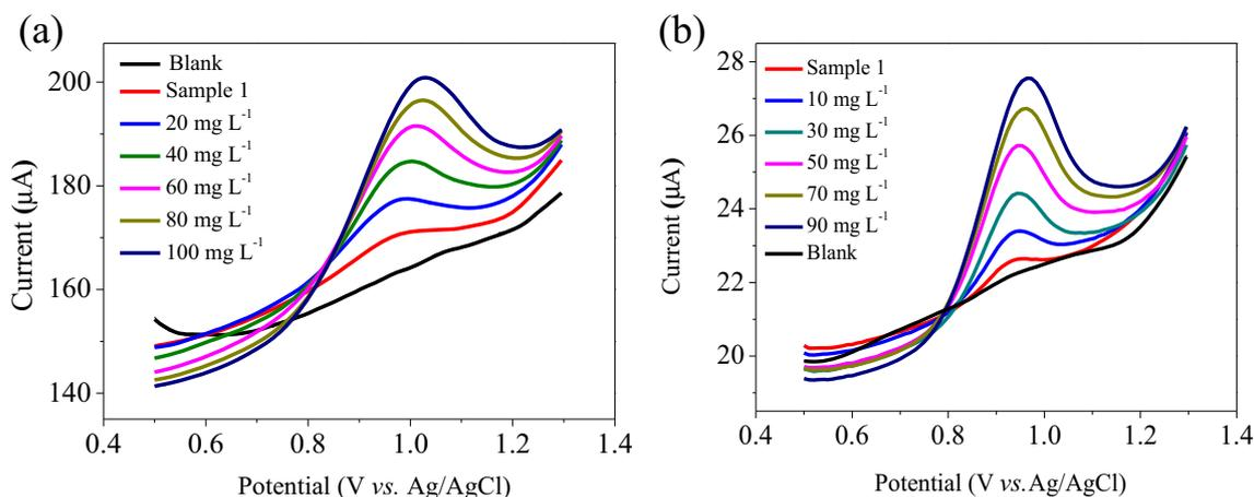
**Figure 11.** Differential pulse voltammogram obtained in the standard addition analysis using the sample with (a) GCE-EG and (b) GCE-CNT in 0.1 mol l<sup>-1</sup> KCl, at pH 10, at 20 mV s<sup>-1</sup>.
