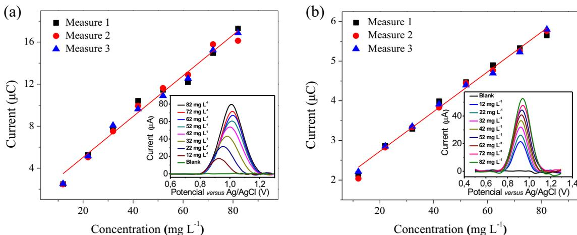
**Figure 8.** Analytical curves were obtained for evaluating the linear range of the morpholine oxidation response in 0.1 mol l<sup>-1</sup> KCl, pH 10 at 20 mV s<sup>-1</sup>, using (a) GCE-EG and (b) GCE-CNT electrodes.
