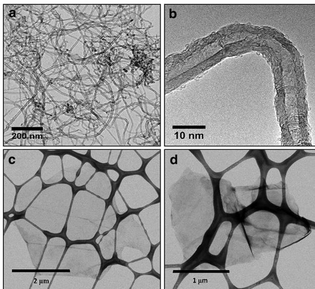
**Figure 1.** (a, b) TEM and HRTEM images, respectively, of CNTs and (c, d) TEM images of EG, on the copper grid covered by a lacy carbon film.
