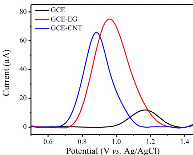
**Figure 7.** Voltammograms obtained by differential pulse voltammetry in the presence of 80 mg l<sup>-1</sup> of morpholine, using GCE, GCE-EG and GCE-CNT, in 0.1 mol l<sup>-1</sup> of KCl (pH 10).
