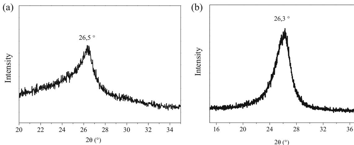
**Figure 5.** X-ray diffraction patterns of (a) EG and (b) CNT samples.
