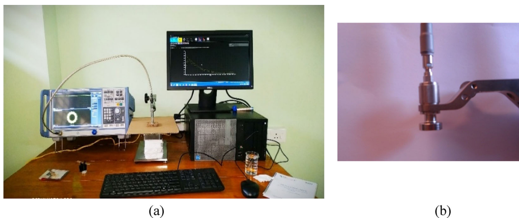
Figure 1. (a) Network analyzer assembly and (b) coaxial probe with flange.
