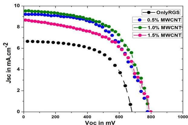
**Figure 7.**  $J$ - $V$  characteristics of MWCNT-RGS based gel electrolytes.
