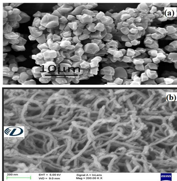
**Figure 5.** SEM images of (a) the isolated starch and (b) MWCNT.
