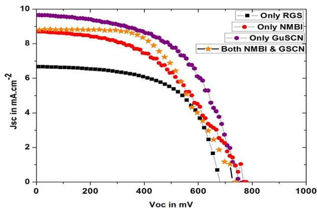
**Figure 6.** Characteristic  $J$ - $V$  curves of DSSCs with RGS/NMBI, RGS/GuNCS and RGS/NMBI+GuNCS electrolytes.
