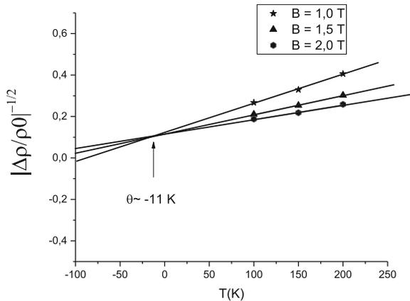
**Figure 2.**  $\left| \left( \frac{\Delta\rho}{\rho_0} \right)^- \right|^{-1/2}$  against temperature  $T$  for different fixed values of magnetic field  $B$ . Deduction of Curie temperature  $\theta$  as indicated by the arrow.
