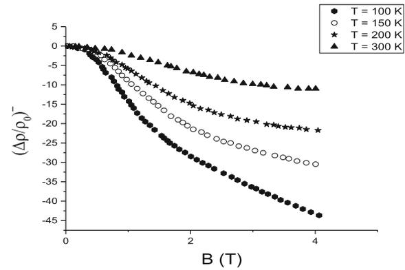
**Figure 1.** Negative magnetoresistance  $\left(\frac{\Delta\rho}{\rho_0}\right)^{-}$  vs. magnetic field up to 4 T at four different temperatures.
