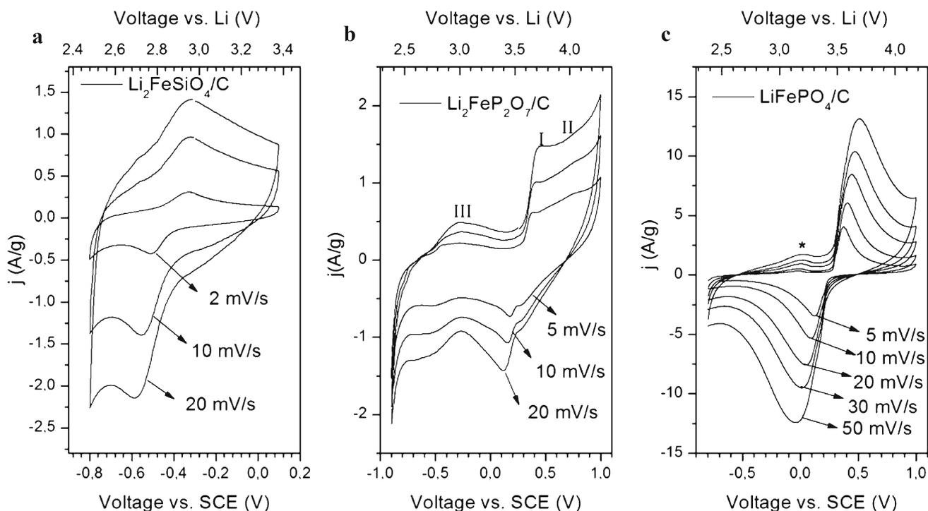
**Figure 4.** Cyclic voltammograms of the obtained composites at various scan rates; the potential vs. Li (top x-axis) is calculated from the measured potential vs. SCE (bottom x-axis) on the basis of reference tables of standard electrode potentials in aqueous solutions vs. normal hydrogen electrode [30].
