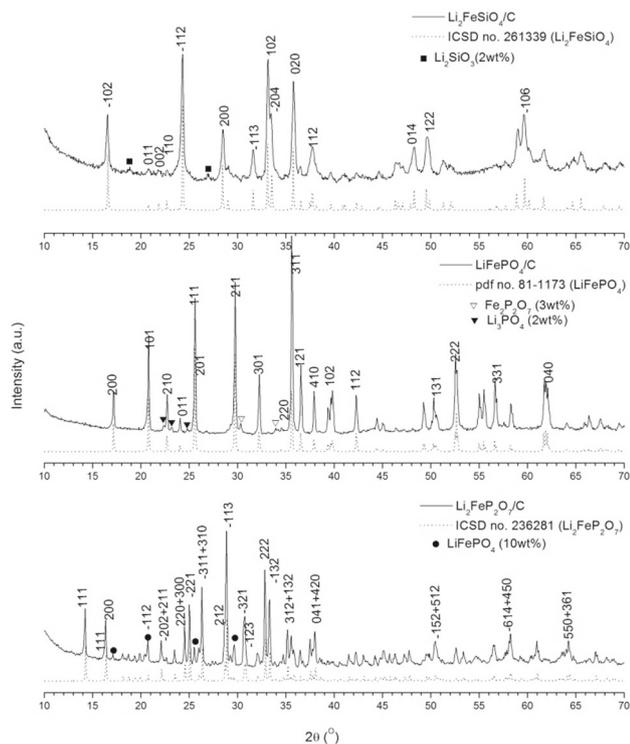
**Figure 3.** X-ray diffraction patterns of the obtained powders (solid line) and corresponding profiles taken from a crystallographic database (dotted line). The most prominent peaks are indexed in  $P2_1/c$  (for  $\text{Li}_2\text{FeSiO}_4$  and  $\text{Li}_2\text{FeP}_2\text{O}_7$ ) and  $Pnma$  ( $\text{LiFePO}_4$ ) symmetry group and observed impurity peaks are marked with a geometrically shaped signs.
