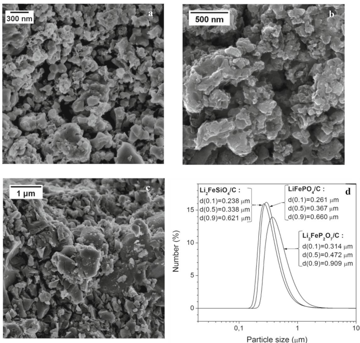
**Figure 2.** SEM micrographs of (a)  $\text{Li}_2\text{FeSiO}_4/\text{C}$ , (b)  $\text{LiFePO}_4/\text{C}$ , (c)  $\text{Li}_2\text{FeP}_2\text{O}_7/\text{C}$  and (d) their particle size distributions.
