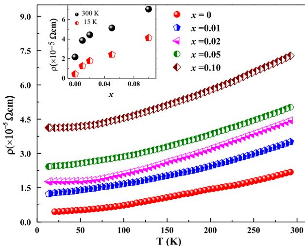
**Figure 2.** Resistivity vs. temperature plots for  $\text{LaNi}_{1-x}\text{Ti}_x\text{O}_3$  ( $x = 0-0.10$ ) thin films on LAO (001). The inset figure shows resistivity vs. doping plot at room temperature, i.e., 300 and 15 K.
