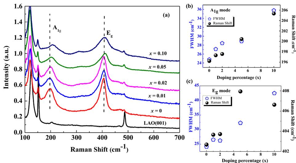
**Figure 4.** (a) Room-temperature Raman spectra of  $\text{LaNi}_{1-x}\text{Ti}_x\text{O}_3$  ( $x = 0-0.10$ ) thin films. (b) The variation of Raman FWHM and peak position of  $A_{1g}$  and  $E_g$  Raman modes with Ti doping percentage in  $\text{LaNi}_{1-x}\text{Ti}_x\text{O}_3$  ( $x = 0-0.10$ ) thin films.
