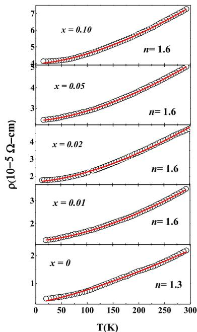
**Figure 3.** Resistivity vs. temperature plots for  $\text{LaNi}_{1-x}\text{Ti}_x\text{O}_3$  ( $x = 0-0.10$ ) thin films on LAO (001). The red line shows the fitting of resistivity using the power law equation.**Table 2.** Transport properties of  $\text{LaNi}_{1-x}\text{Ti}_x\text{O}_3$  ( $x = 0-0.10$ ) thin films deposited on LAO.
