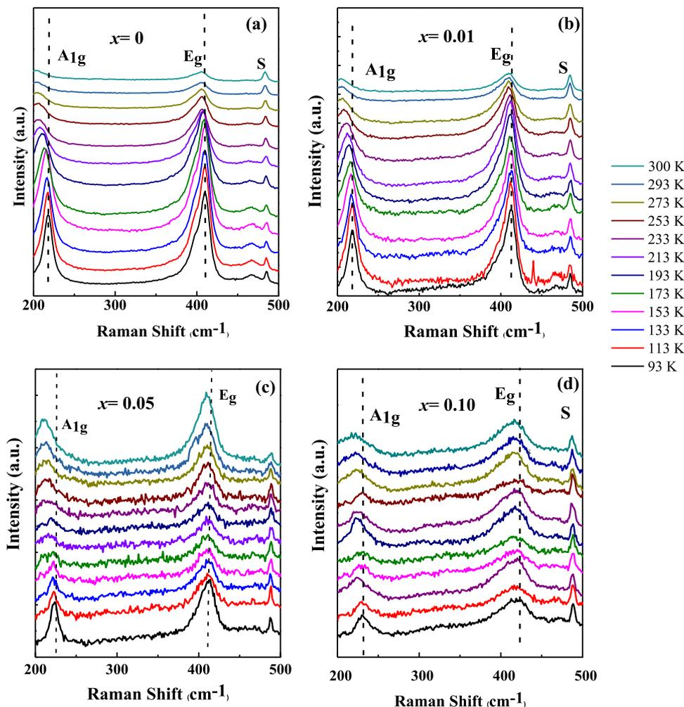
**Figure 5.** (a–d) Temperature-dependent Raman spectra of  $\text{LaNiO}_3$ ,  $\text{LaNi}_{0.99}\text{Ti}_{0.01}\text{O}_3$ ,  $\text{LaNi}_{0.95}\text{Ti}_{0.05}\text{O}_3$  and  $\text{LaNi}_{0.90}\text{Ti}_{0.10}\text{O}_3$  thin films, respectively.
