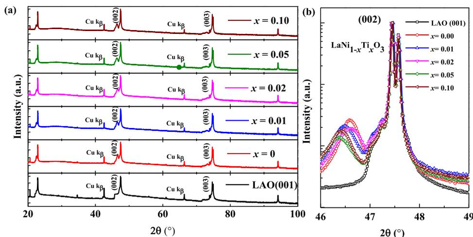
**Figure 1.** (a) X-ray diffraction patterns of  $\text{LaNi}_{1-x}\text{Ti}_x\text{O}_3$  ( $x = 0-0.10$ ) thin films grown on LAO (001) substrate. (b) Enlarged view of (002) Bragg's diffraction of  $\text{LaNi}_{1-x}\text{Ti}_x\text{O}_3$  ( $x = 0-0.10$ ) thin films.
