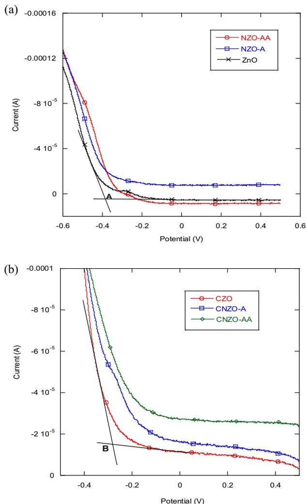
**Figure 7.**  $I$ - $V$  curves of linear potential scan in a potential range to determine the  $E_c$  values for (a) NZO and (b) CNZO samples.
