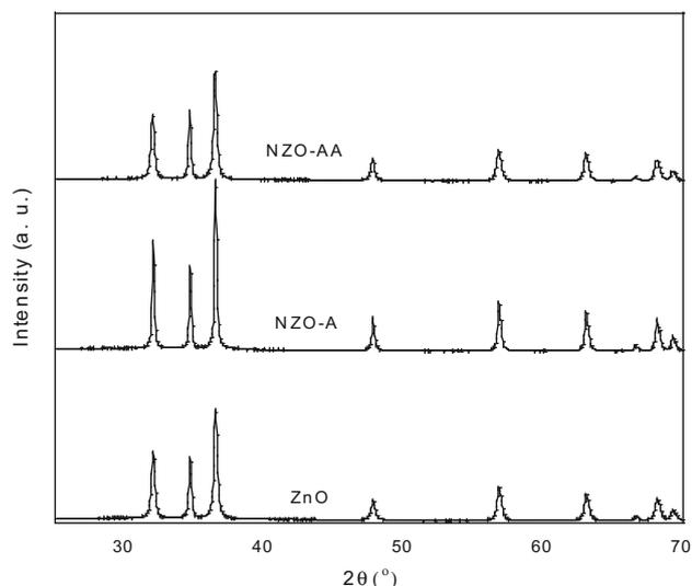
**Figure 1.** XRD patterns for the N-doped ZnO (NZO) samples.
