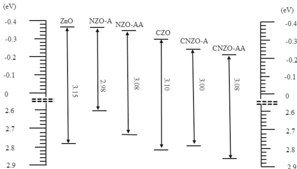
**Figure 8.** Energy band diagram for various Cu and N doping in ZnO samples.
