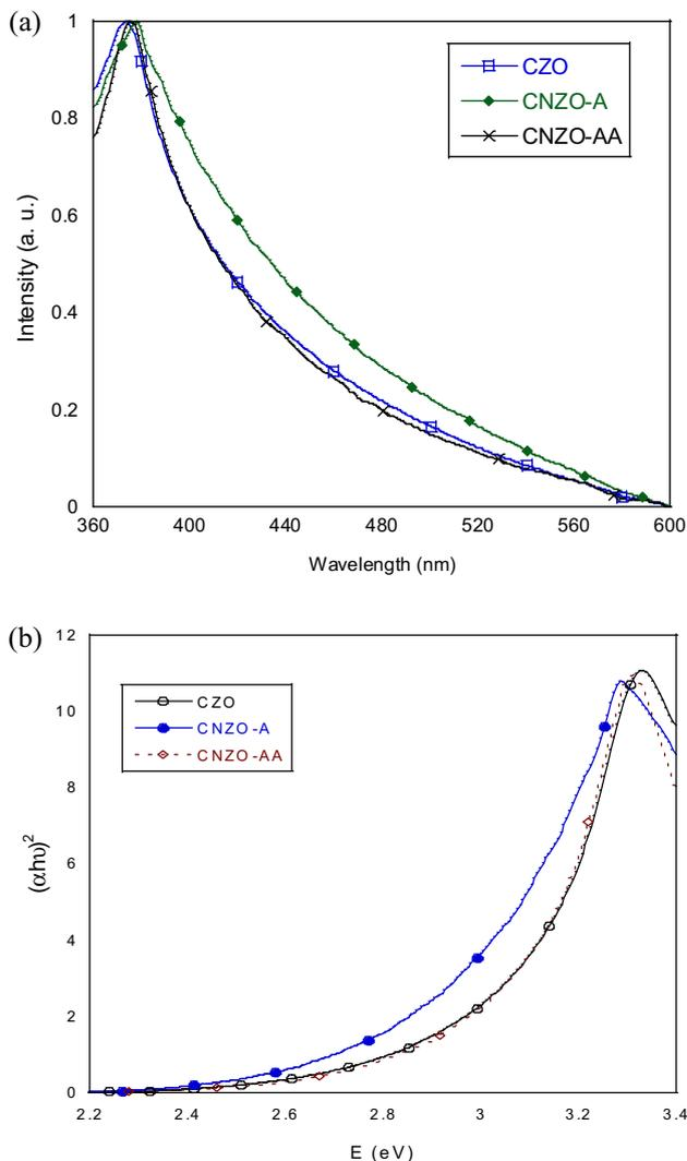
**Figure 5.** Plots of (a) UV-vis spectra and (b)  $(\alpha hv)^{1/2}$  vs. photonic energy ( $\tau$ -plot) for the Cu- and N-doped ZnO samples.
