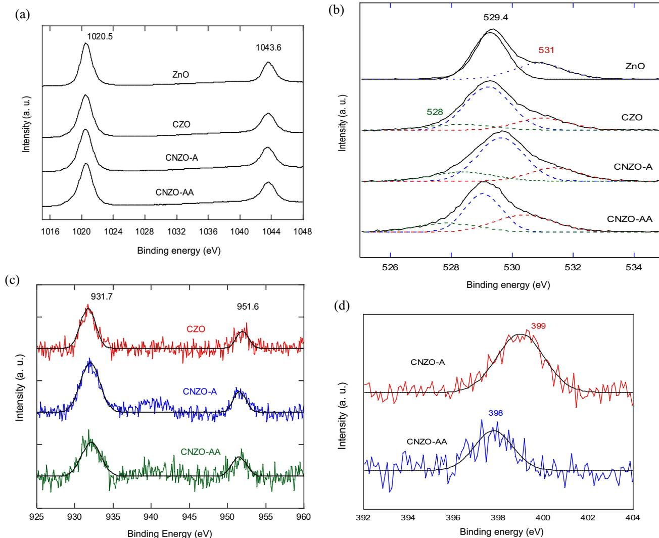
**Figure 6.** Core-level spectra of (a) Zn 2p, (b) O 1s, (c) Cu 2p and (d) N 1s for the doped ZnO samples by XPS survey.
