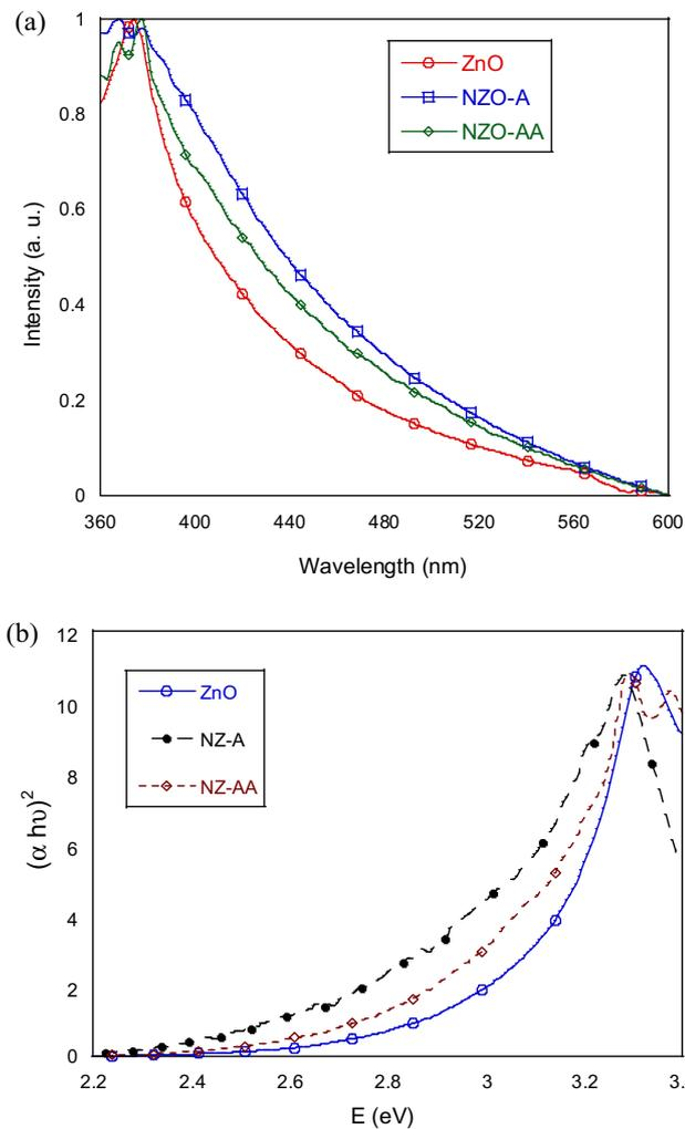
**Figure 3.** Plots of (a) UV-vis spectra and (b)  $(\alpha hv)^{1/2}$  vs. photonic energy ( $\tau$ -plot) for the NZO samples.
