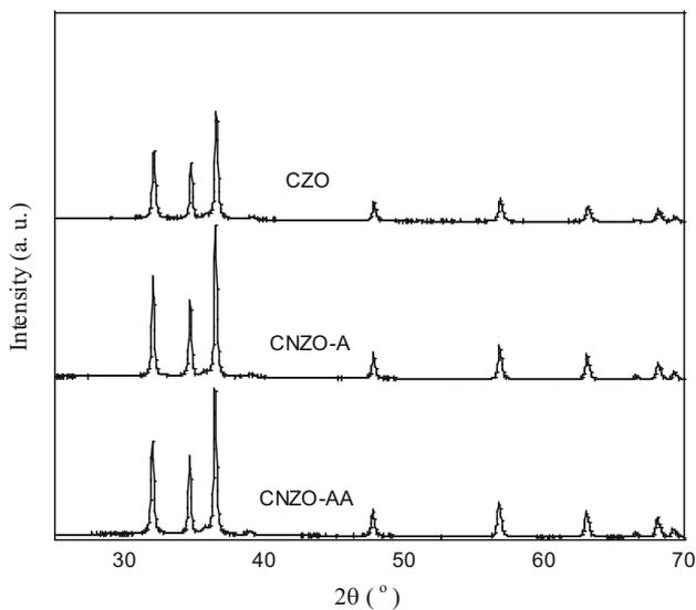
**Figure 4.** XRD patterns for the Cu- and N-doped ZnO samples.
