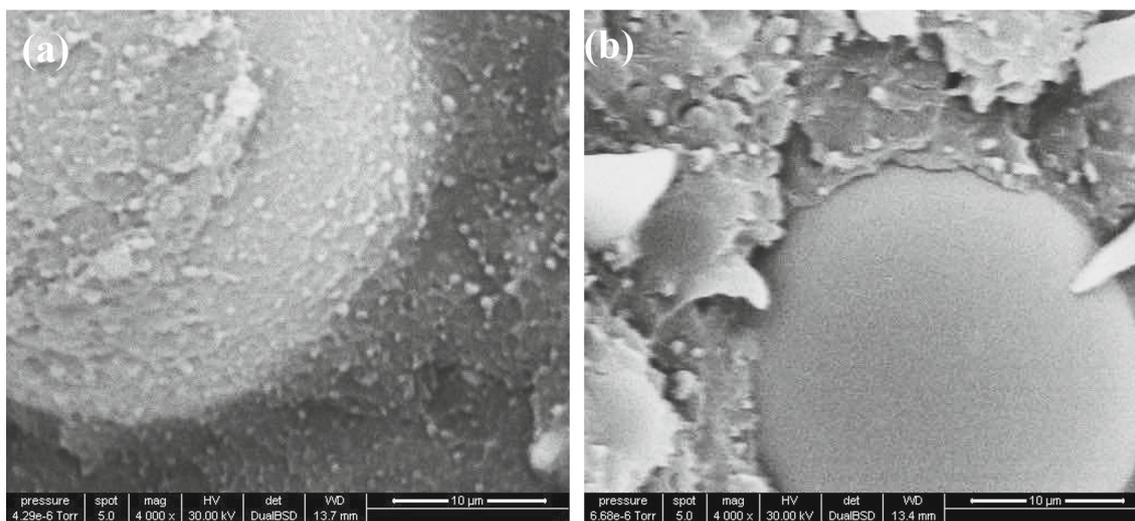
**Figure 5.** Representative SEM images of interfaces from PPE/PA66 composites using (a) surface-treated S38XHS and (b) untreated S38XHS grade of HGB.
