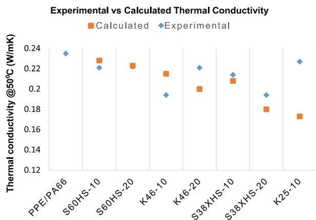
**Figure 3.** Graphical depiction of the experimental and calculated thermal conductivities of different samples.
