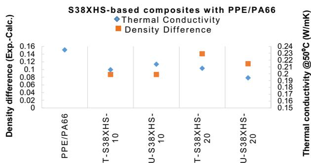
**Figure 4.** Plot of the density difference vs. thermal conductivity plot for S38XHS-based PPE/PA66 composites.
