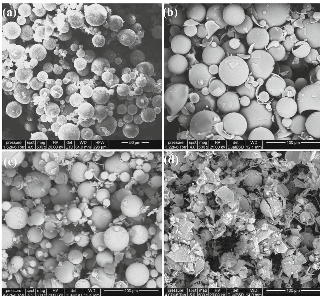
**Figure 2.** SEM images showing the HGB breakage for composite with (a) 10 wt% S60HS, (b) 10 wt% K46, (c) 10 wt% S38XHS and (d) 10 wt% K25.
