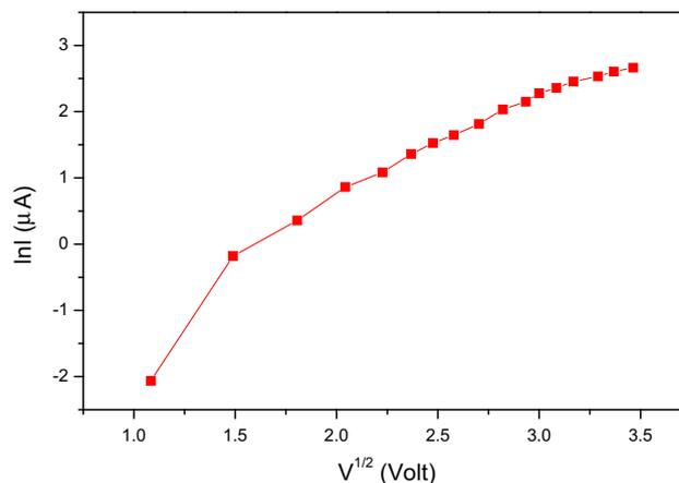
**Figure 6.**  $\ln I$  vs.  $V^{1/2}$  plot for indigo dye-based diode.
