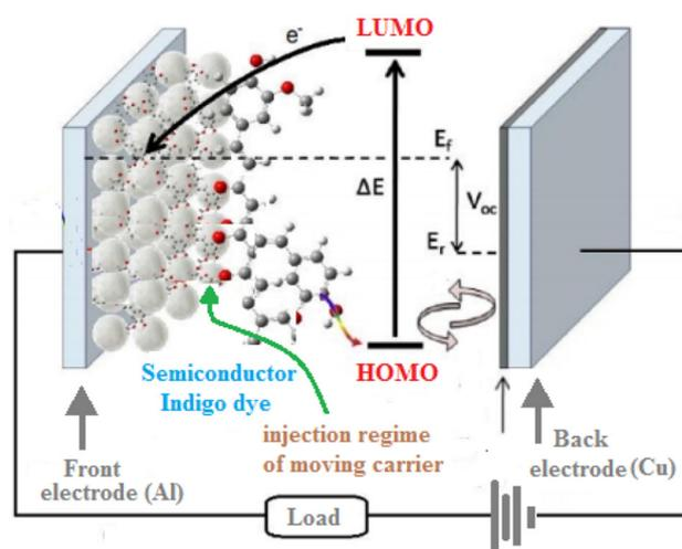
**Figure 2.** Dark current measurement setup where Al and Cu have been used as front and back electrodes, respectively, whereas the indigo dye has been selected as active layer sandwiched between the electrodes [6].
