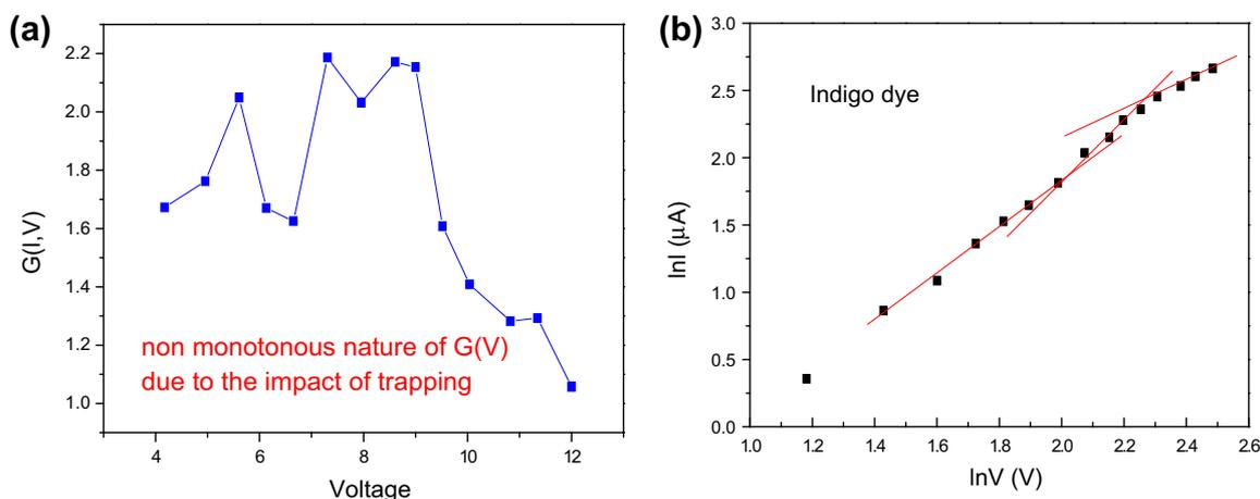
**Figure 4.** (a)  $G(V)$ - $V$  plot of indigo dye-based diode. Multiple distortions in the figure explain the presence of multiple discrete traps. The first in the plot is quite suppressed and is generated due to  $V_{bi}$ . Remaining peaks arise from other deeper traps; and (b)  $\log I$ - $\log V$  plot for indigo dye-based device used to calculate trap energy.
