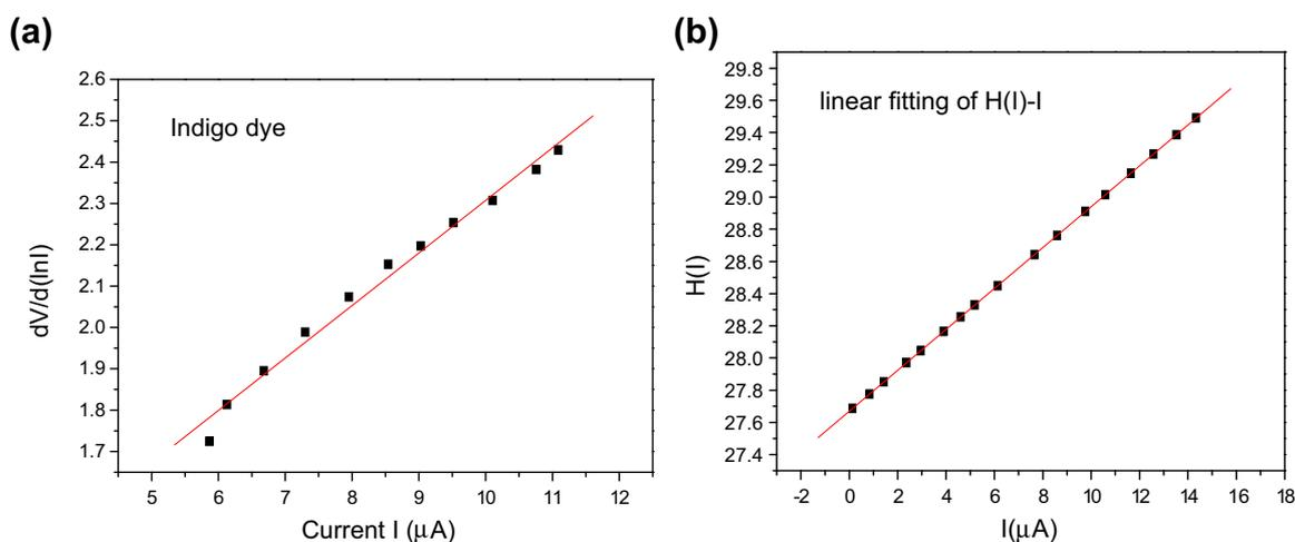
**Figure 5.** (a)  $(dV/d \ln I)$ - $I$  plot and (b)  $H(I)$ - $I$  plot of indigo dye-based diode.
