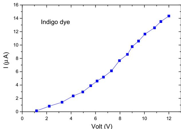
Figure 3. *I*–*V* Characteristics of indigo dye-based diode.
