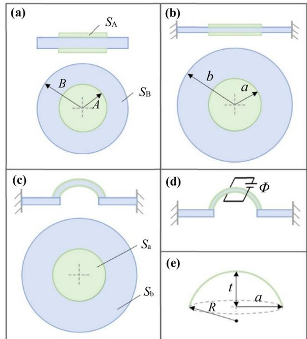
**Figure 5.** The deformation of a tunable solid-body lens. (a) Reference state. (b) Pre-stretched state. (c) Resting state. (d) Actuated state. (e) Representation of the lens as a spherical cap that has a cap height  $t$ , a base diameter  $2a$ , and the radius of curvature  $R$ .
