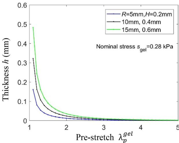
**Figure 2.** Theoretical prediction of the stretch using constant nominal stress for the PAM hydrogel with different original thicknesses and radii.
