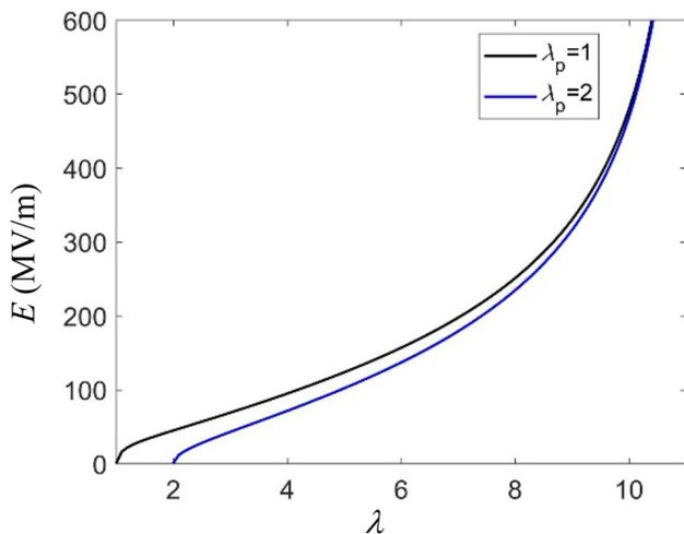
**Figure 4.** The predicted curves between electric field and stretch. Different levels of pre-stretches from  $\lambda_p = 1$  to 2 were imposed to the DE actuator coupling the PAM hydrogel.
