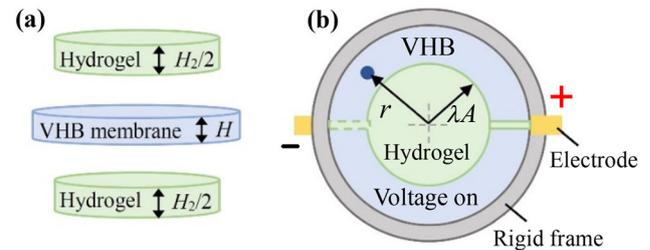
**Figure 3.** The schematic of an actuator made of a DE sandwiched between hydrogels. (a) In the reference state, a circular DE membrane with thickness  $H$ , the combined thickness of the two hydrogel films is  $H_2$ . (b) In an actuated state, a material particle is marked by radius  $r$  that changes from reference  $R$ , and the radius of the active region moves to  $\lambda A$  from reference  $A$ .
