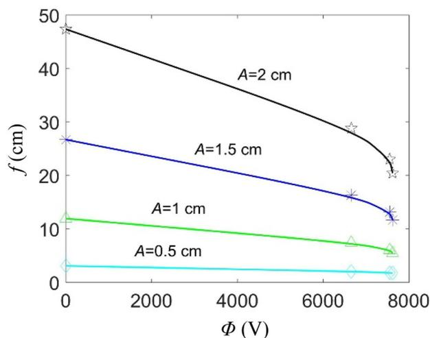
**Figure 6.** Variations of the lens focal length with the applied voltage.
