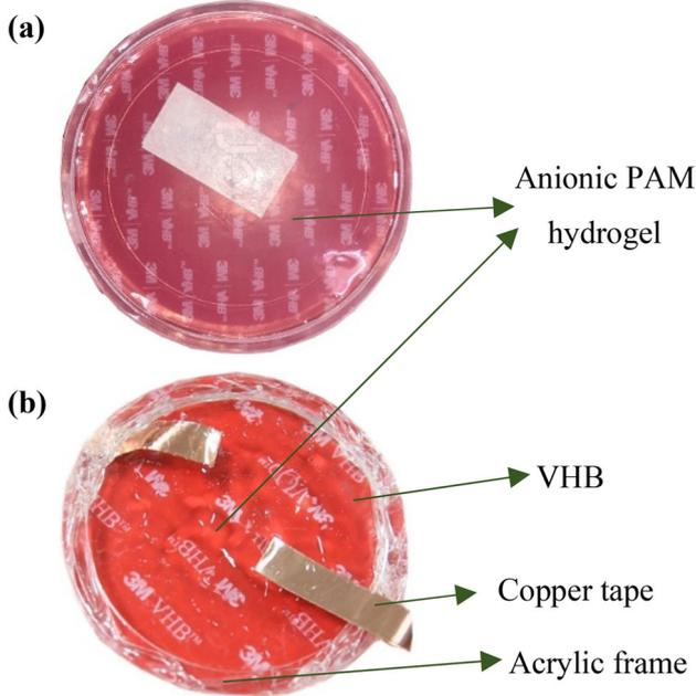
**Figure 1.** (a) The PAM hydrogel containing NaCl is highly transparent and flexible. (b) An actuator for a tunable lens that consists of a frame, a thin DE membrane (the pre-stretch  $\lambda_p = 1$ , the thickness  $H = 0.5$  mm) with hydrogel electrodes.
