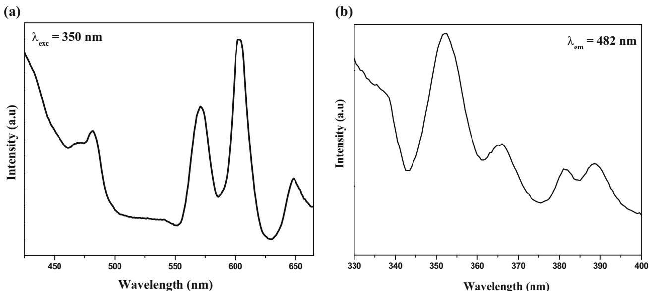
**Figure 4.** (a) Emission and (b) excitation spectra of spin-coated  $\text{CaZr}_{0.9}\text{Sm}_{0.025}\text{Dy}_{0.075}\text{O}_3$  film.
