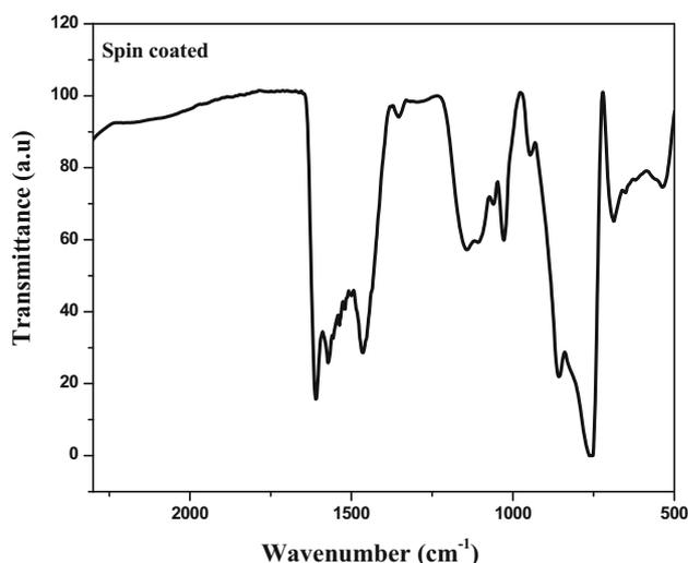
**Figure 2.** FTIR spectrum of spin-coated  $\text{CaZr}_{0.9}\text{Sm}_{0.025}\text{Dy}_{0.075}\text{O}_3$  film.
