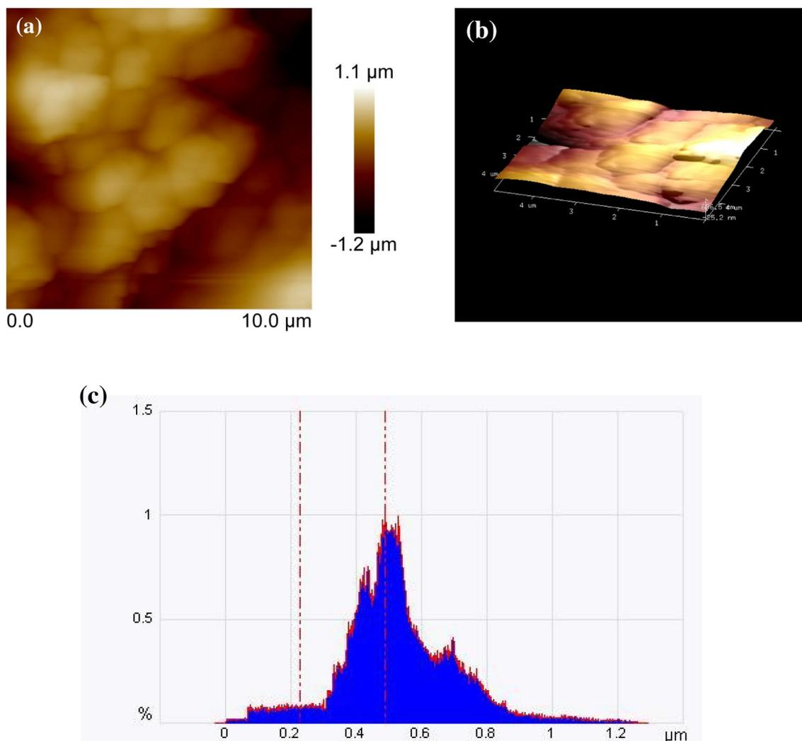
**Figure 3.** (a and b) AFM micrographs for the deposited film. (c) Depth profiling for deposited film.
