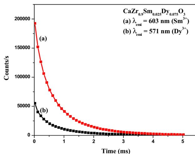
**Figure 5.** Decay curves of  $\text{CaZr}_{0.9}\text{Sm}_{0.025}\text{Dy}_{0.075}\text{O}_3$  film.
