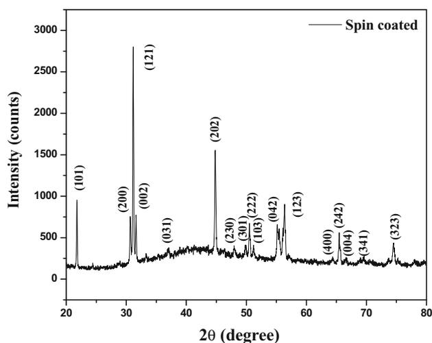
**Figure 1.** XRD pattern of spin-coated  $\text{CaZr}_{0.9}\text{Sm}_{0.025}\text{Dy}_{0.075}\text{O}_3$  film.
