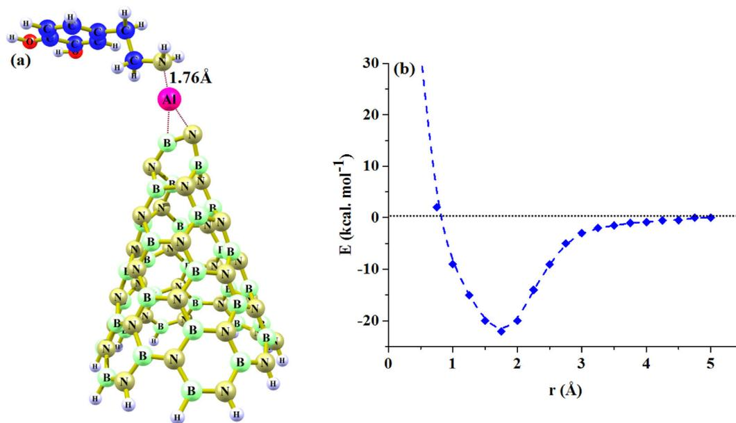
**Figure 4.** (a) Optimized structure DA and Al-BNNCs complex and (b) adsorption energy curves obtained by vertical scanning of intermolecular distances (0.5–5 Å) between DA and Al-BNNCs.
