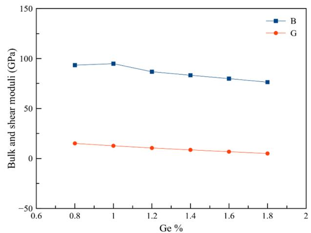
**Figure 3.** Bulk ( $B$ ) and shear ( $G$ ) moduli of Ti–15Nb– $x$ Ge alloys.
