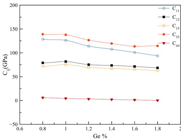
**Figure 2.** Elastic stiffness constants of Ti–15Nb– $x$ Ge alloys.
