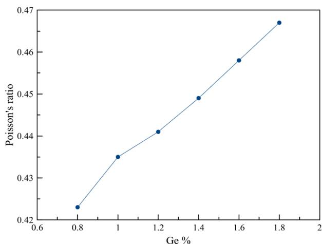
Figure 6. Poisson's ratio of Ti-15Nb-xGe alloys.
