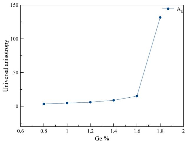
Figure 7. Universal anisotropy parameters of Ti-15Nb-xGe alloys.
