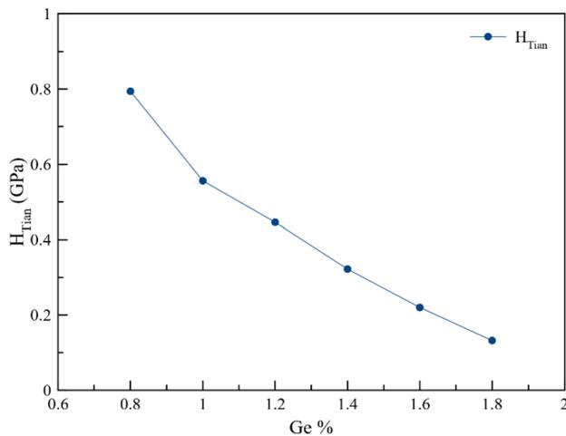
**Figure 8.** Hardness values of Ti–15Nb–xGe alloys.
