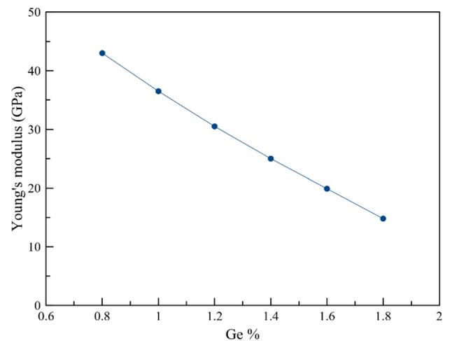
**Figure 4.** Young's modulus ( $E$ ) of Ti–15Nb– $x$ Ge alloys.
