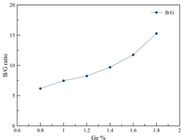
Figure 5. Ductile behaviour of Ti-15Nb-xGe alloys.
