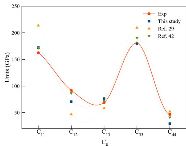
**Figure 1.** Elastic stiffness constants of  $\alpha$ -Ti.
