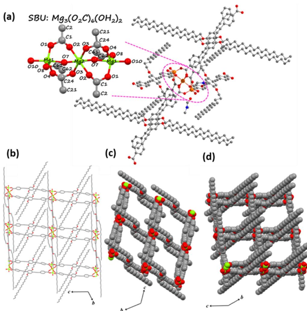
**Figure 1.** Single crystal structure of **1**: (a) asymmetric unit showing the coordination of OPE dicarboxylates around the Mg centres. Inset: representation of the  $Mg_3(O_2C)_6(OH_2)_2$  SBU showing the coordination environment around Mg centres. (b) View showing the 2D grid formation. (c) Spacefill model view of the pores formed in the 2D grid. (d) Spacefill model showing the surface projected alkyl chains in the 2D grid. (Solvent molecules have been omitted for clarity.)
