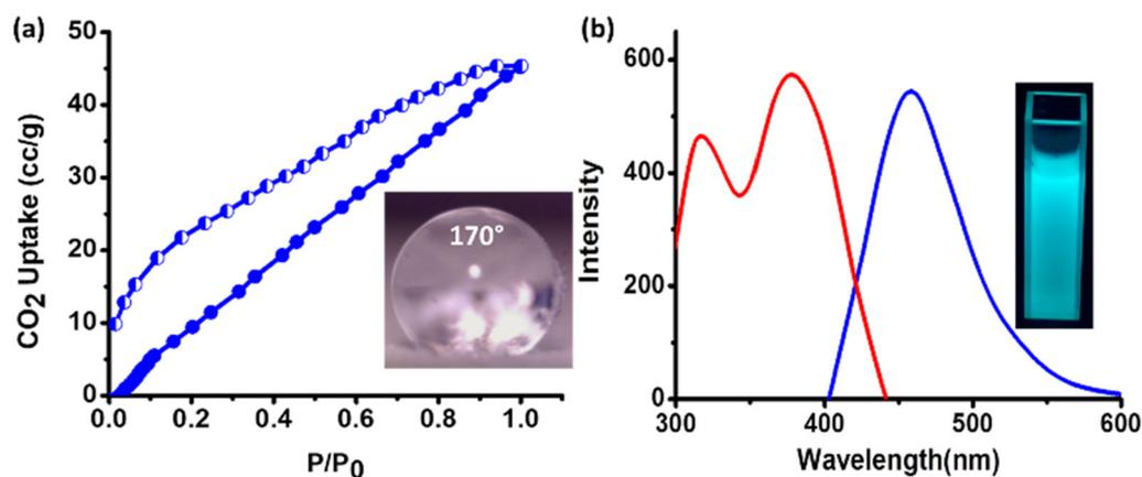
**Figure 2.** (a)  $CO_2$  adsorption isotherm at 195 K for **1**. Inset: water contact angle image on **1** coated glass substrate. (b) PL plot of **1** in THF dispersed state. Inset: image of **1** dispersed in THF under UV.
