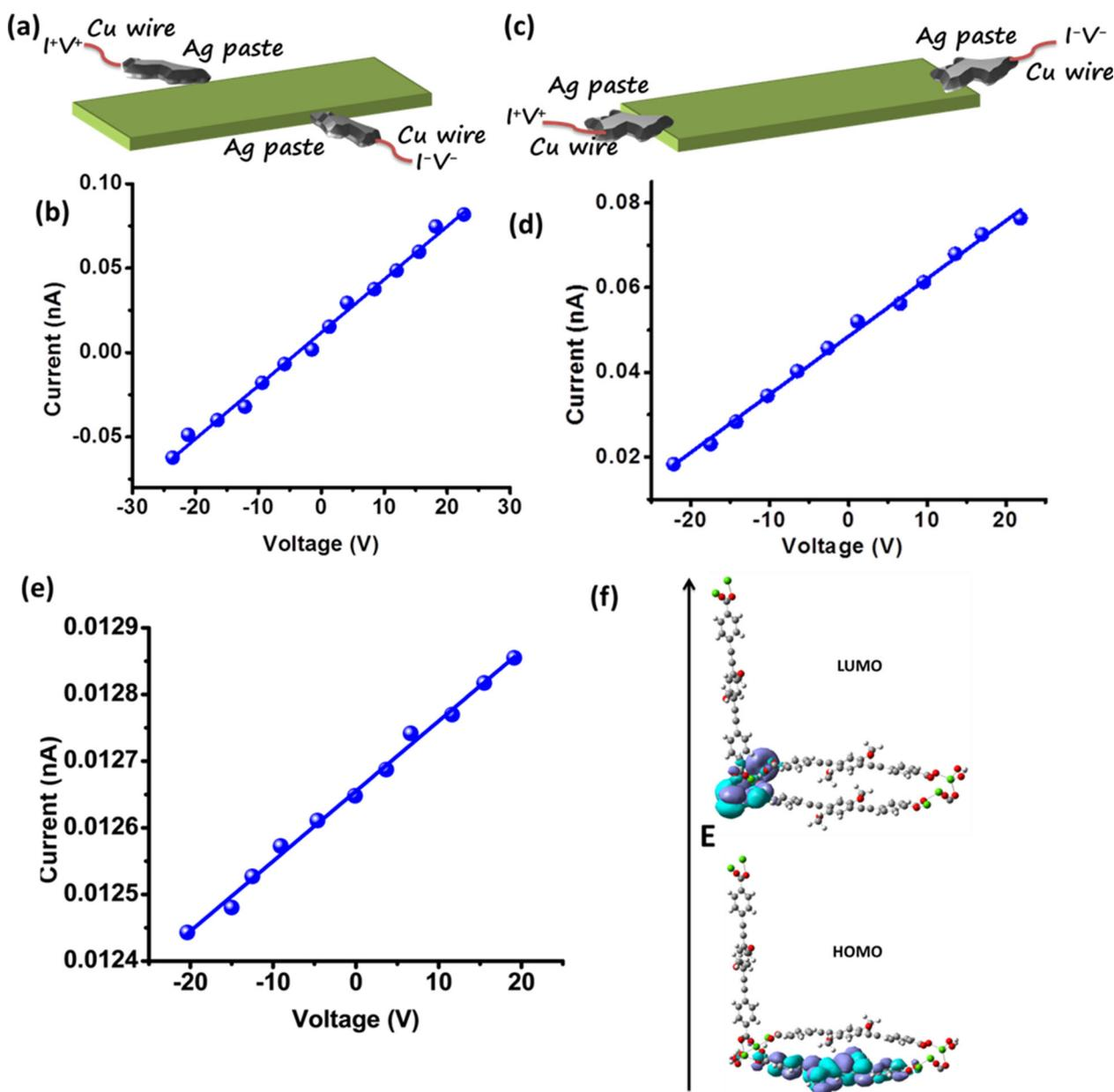
**Figure 3.** Schematic showing the experimental setup used for measurement of  $I$ - $V$  characteristics of (a) side face, (c) broad face of **1** single crystals of **1**.  $I$ - $V$  plots for (b) side face, (d) broad face of **1** single crystals, (e) thin film of **1** and (f) HOMO (lower) and LUMO (upper) plots for **1** shown using a fragmented unit for pictorial clarity.
