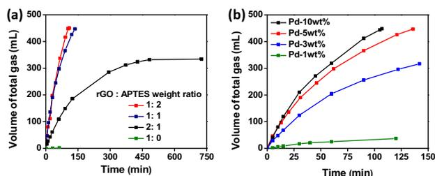
**Figure 2.** HCOOH decomposition at room temperature with (a) 5 wt% palladium loaded on different APTES-functionalized GO support and (b) rGO:APTES (1:1) as support by varying the palladium content. All the experiments were performed with 10 ml, 1 M HCOOH and 50 mg catalyst ( $n_{Pd}/n_{HCOOH} = 0.002$ ).
