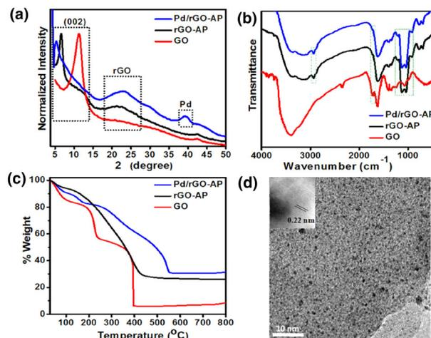
**Figure 1.** Characterization of GO, rGO-AP and Pd/rGO-AP by (a) PXRD, (b) FTIR, (c) TGA and (d) TEM (inset shows the interlayer distance of Pd (111) plane).
