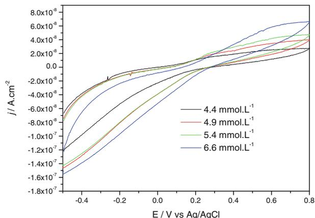
**Figure 8.**  $\text{V}_2\text{O}_5/\text{GOx}$  voltammograms, in  $0.1 \text{ mol l}^{-1}$  PBS buffer, pH 6,  $v = 20 \text{ mV s}^{-1}$ , with varying concentrations of glucose.
