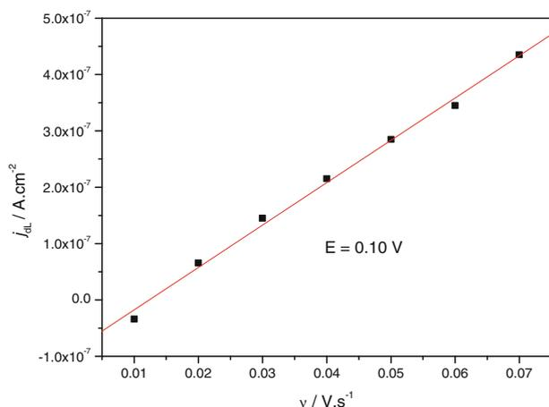
**Figure 7.** Variation of current density in double layer region as a function of scan rate.
