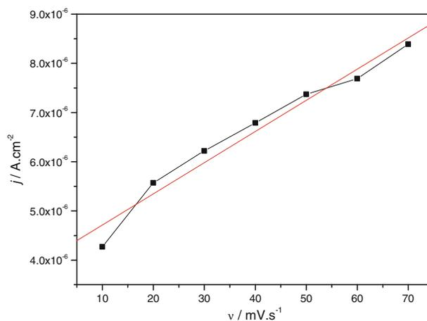
**Figure 6.** Dependence of current density as a function of scan rate. The values were collected on transition region.
