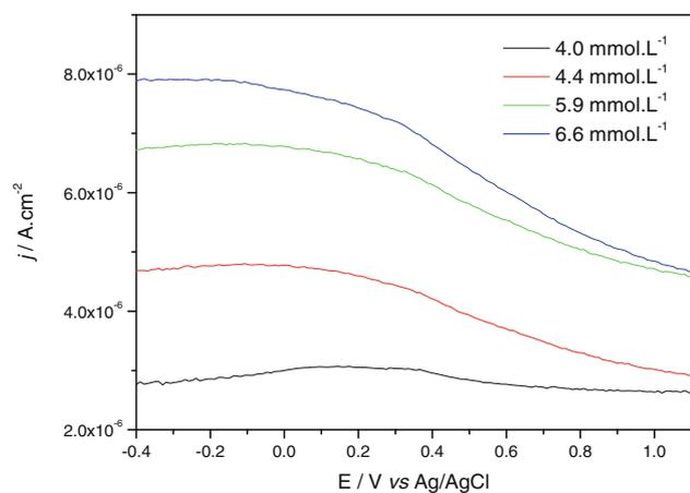
**Figure 10.** Square wave voltammogram using  $V_2O_5/GOx$ , in PBS, pH = 6,  $\nu = 20 \text{ mV s}^{-1}$ , depending on the variation in glucose concentrations.
