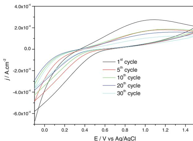
**Figure 1.** Cyclic voltammogram of the  $V_2O_5$  film obtained during the 30 cycles before GOx immobilization,  $\nu = 20\text{ mV s}^{-1}$ , PBS,  $\text{pH} = 6$ , glucose  $4.4\text{ mmol l}^{-1}$ .
