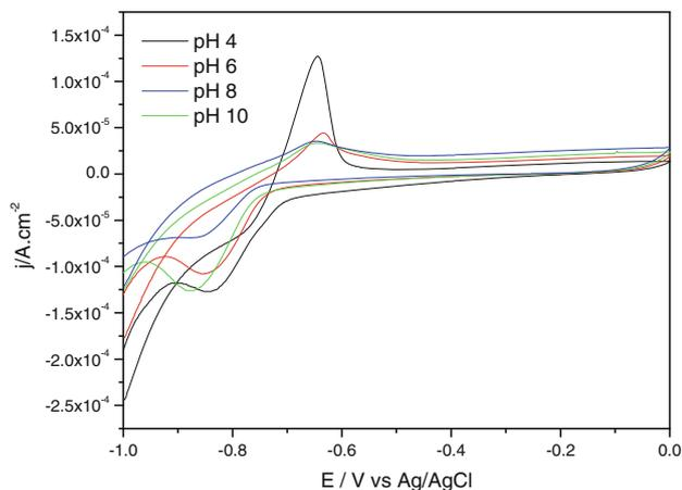
**Figure 3.** V<sub>2</sub>O<sub>5</sub>/GOx voltammograms, in 0.1 mol l<sup>-1</sup> PBS buffer, with 4.4 mol l<sup>-1</sup> glucose,  $\nu = 20 \text{ mV s}^{-1}$ , with pH range 4 to 10.
