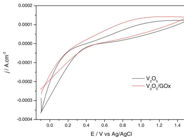
**Figure 2.** Cyclic voltammograms of  $V_2O_5$  and  $V_2O_5/\text{GOx}$ ,  $\nu = 20\text{ mV s}^{-1}$ , PBS,  $\text{pH} = 6$ , glucose  $4.4\text{ mmol l}^{-1}$ .
