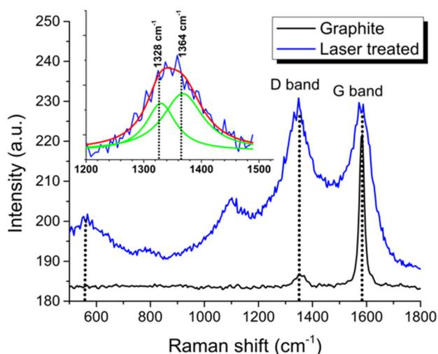
**Figure 5.** Raman analysis of graphite (black) and laser processed sample (blue). The deconvoluted peaks (green) shown in inset differentiates the diamond peak at  $1328\text{ cm}^{-1}$  from graphitic D band.
