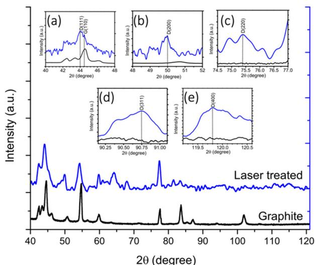
**Figure 3.** XRD diffractogram of graphite sample (in black) and laser-treated sample (in blue). In inset (a–e), high-resolution XRD of laser-treated sample showing diamond planes (111), (200), (220), (311) and (400), corresponding at  $2\theta = 44.1, 50, 75.4, 90.7$  and  $119.8$ , respectively.
