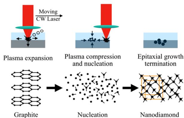
**Figure 2.** Schematic of phase transformation from graphite to nanodiamond. During irradiation of graphitic target plasma expands. Post irradiation rapid compression of plasma plume takes place. The rapid compression promotes epitaxial growth on diamond nucleation site.
