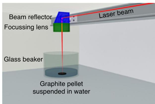
**Figure 1.** Graphical illustration of experimental setup.
