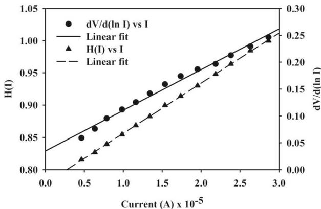
Figure 3.  $d(V)/d(\ln I)$  and  $H(I)$  variations with respect to observed Schottky diode current.
