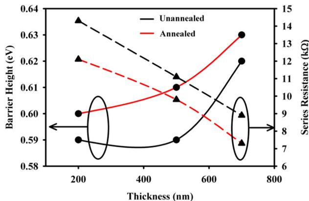
**Figure 4.** Variations in barrier height and series resistance as a function of CIAS film thickness, calculated using Cheung's function.
