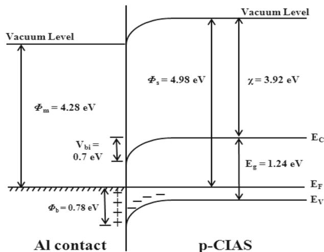
**Figure 7.** Energy band diagram of Al/p-CIAS Schottky diode.
