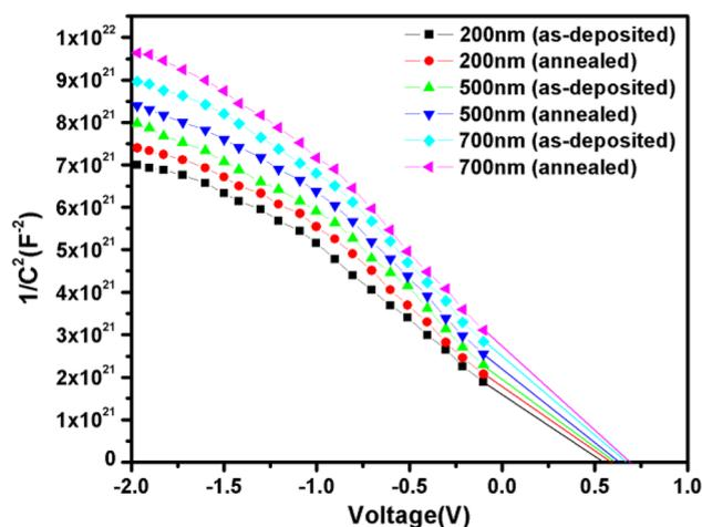
**Figure 6.**  $1/C^2-V$  characteristics of as-deposited and annealed Al/p-CIAS Schottky diodes.
