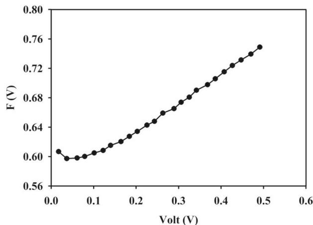
**Figure 5.** Norde's  $F(V)$  variation with respect to applied voltage ( $V$ ) for the Schottky diodes.
