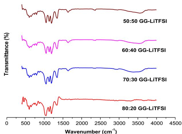
**Figure 1.** FTIR spectra of pure GG, LiTFSI and GG–LiTFSI polymer electrolytes.
