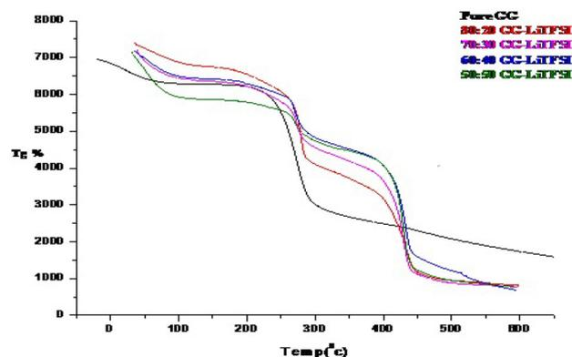
**Figure 3.** TG curve of pure GG and GG–LiTFSI polymer electrolytes.
