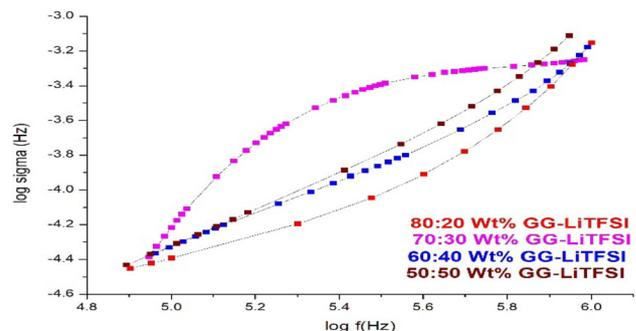
**Figure 6.** Conductance spectra of GG–LiTFSI polymer electrolytes.
