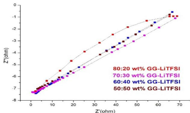
**Figure 5.** Cole–Cole plot for GG–LiTFSI polymer electrolytes.
