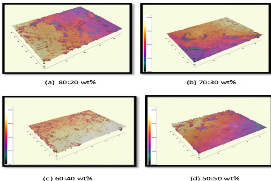
**Figure 4.** Zeta 3D images of GG–LiTFSI polymer electrolytes.
