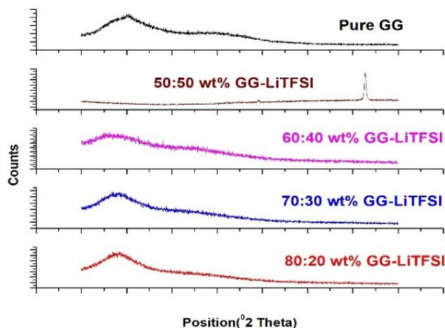
**Figure 2.** XRD pattern of pure GG and GG–LiTFSI polymer electrolytes.
