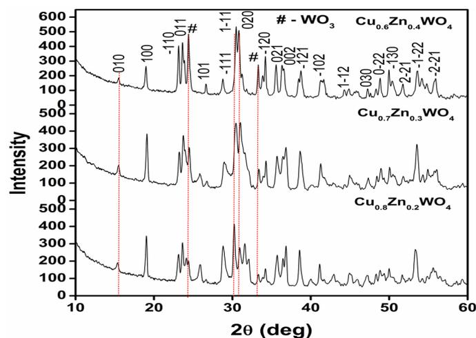
Figure 1. XRD pattern of  $\text{Cu}_{1-x}\text{Zn}_x\text{WO}_4$  nanoparticles.
