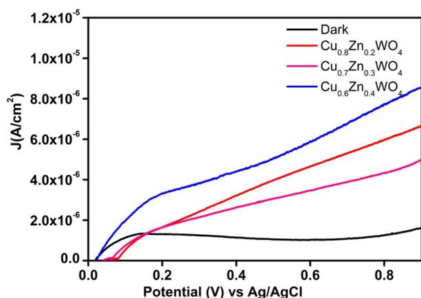
**Figure 4.** J-V curve of  $\text{Cu}_{1-x}\text{Zn}_x\text{WO}_4$  nanoparticles.
