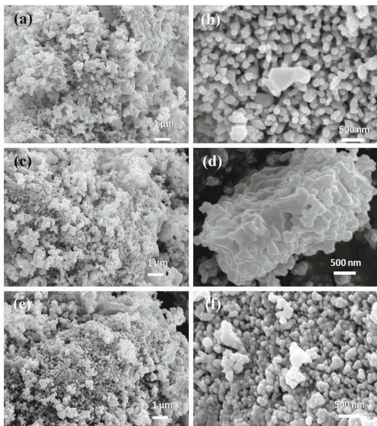
**Figure 2.** SEM images of  $\text{Cu}_{1-x}\text{Zn}_x\text{WO}_4$  nanoparticles: (a and b)  $x = 0.2$ , (c and d)  $x = 0.3$ , (e and f)  $x = 0.4$ .
