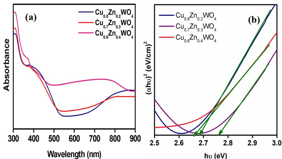
**Figure 3.** (a) UV-Vis spectra and (b) Tauc plot of  $\text{Cu}_{1-x}\text{Zn}_x\text{WO}_4$  nanoparticles.
