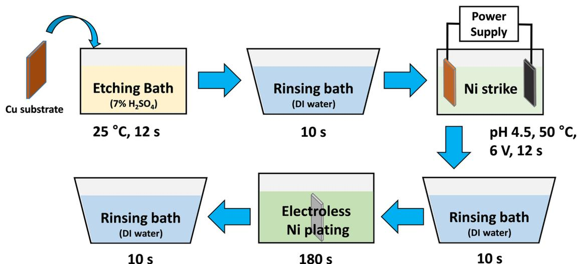
**Figure 1.** Technical flow chart of Ni–B electroless plating.
