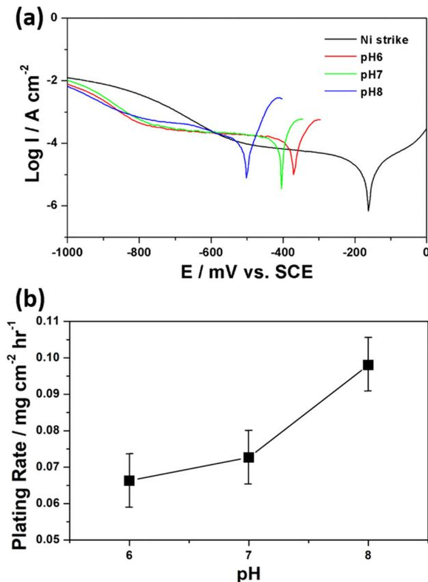
Figure 3. Effect of varying pH values on (a) polarization curves and (b) electroplating rates.
