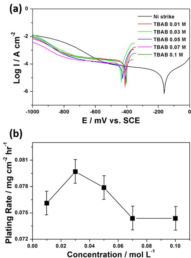
Figure 2. Effect of varying TBAB concentrations on (a) polarization curves and (b) electroplating rates.
