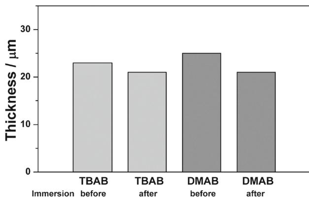
**Figure 4.** Comparison of thickness of Ni–B plating samples using TBAB and DMAB before and after immersion in the electrolyte.
