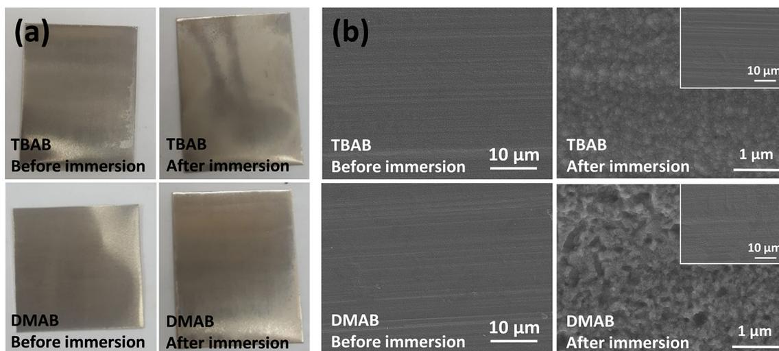
**Figure 5.** Comparison of (a) optical and (b) SEM images of Ni–B plating samples using TBAB and DMAB before and after immersion in the electrolyte.
