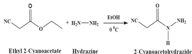
**Scheme 1.** Preparation scheme of 2-cyanoacetohydrazide.
