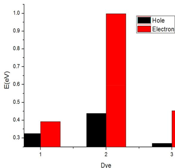
**Figure 4.** Hole and electron reorganization energies of dye-1 (CHMA), dye-2 (CDBA) and dye-3 (AMCH) in eV at the B3LYP/6-31G\*\* level of theory.
