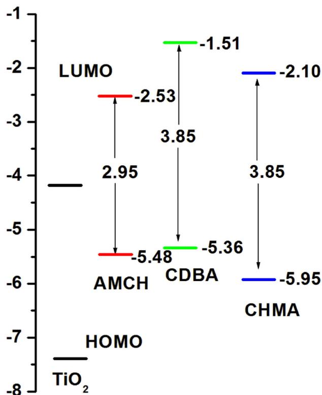
**Figure 3.** HOMO and LUMO energy level, energy gap of all prepared dyes obtained from DFT calculation and energy levels analogous to the valence and conduction band of  $\text{TiO}_2$ .
