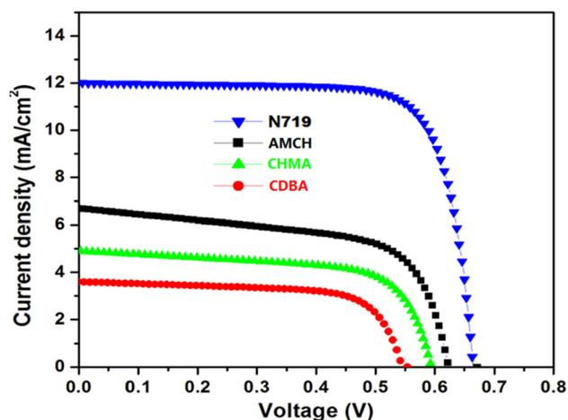
**Figure 5.** Current–voltage characteristics of DSSCs based on (a) dye (CHMA), (b) dye (CDBA), (c) dye (AMCH) and (d) N719 commercial dye (area: 1 cm<sup>2</sup>).
