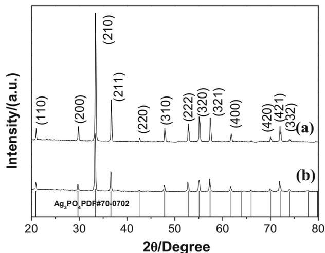
**Figure 2.** XRD patterns of the  $\text{Ag}_3\text{PO}_4$  sample at the same reaction temperature and time: (a) with PEG and (b) without PEG.
