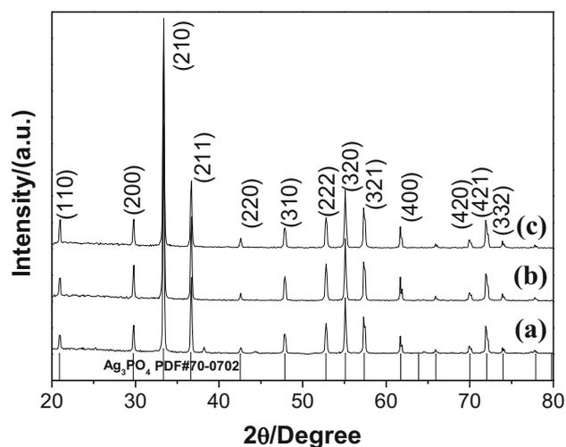
**Figure 1.** XRD patterns of the  $\text{Ag}_3\text{PO}_4$  sample at different temperatures: (a)  $120^\circ\text{C}$ , (b)  $150^\circ\text{C}$  and (c)  $180^\circ\text{C}$ .
