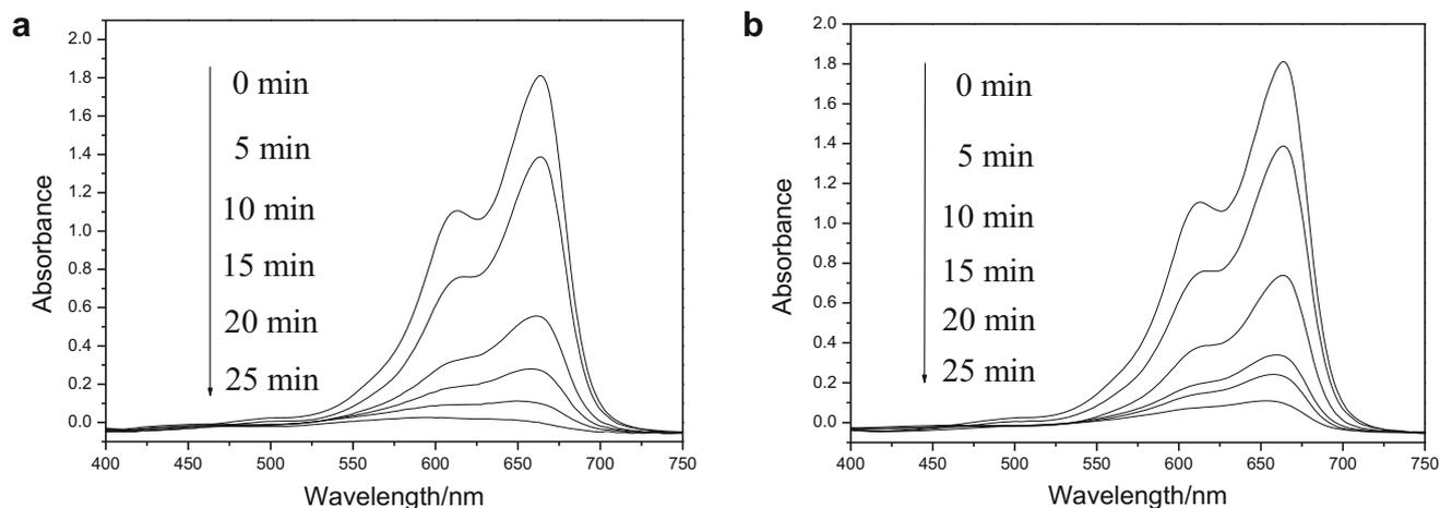
**Figure 5.** UV-visible absorption spectra of photocatalytic degradation for an aqueous solution of MB on  $\text{Ag}_3\text{PO}_4$  sample: (a) with PEG and (b) without PEG.
