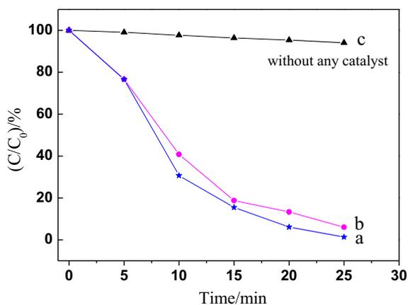
**Figure 6.** Photodegradation curves of MB: (a) with PEG and (b) without PEG.
