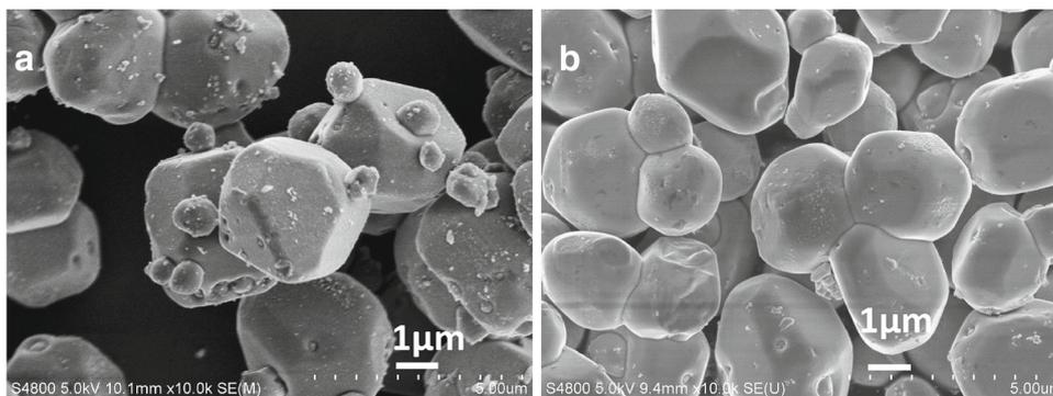
**Figure 4.** SEM patterns of the  $\text{Ag}_3\text{PO}_4$  sample: (a) with PEG and (b) without PEG.
