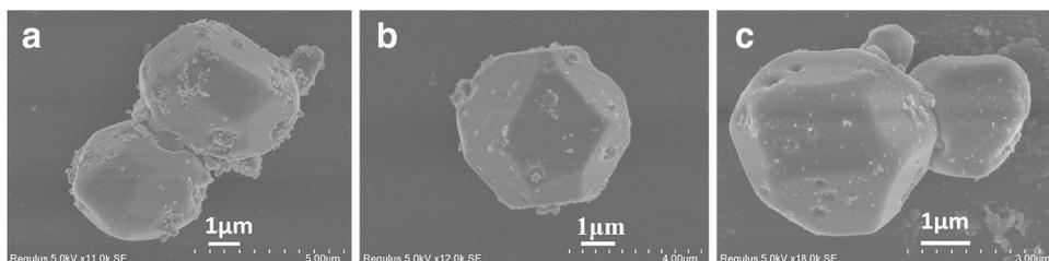
**Figure 3.** SEM patterns of the  $\text{Ag}_3\text{PO}_4$  sample at different temperatures: (a) 120°C, (b) 150°C and (c) 180°C.
