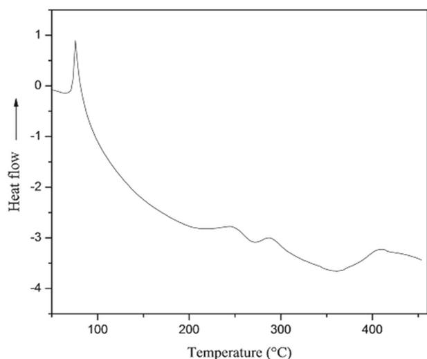
**Figure 5.** DSC thermogram of ibuprofen-based hyperbranched polyester.
