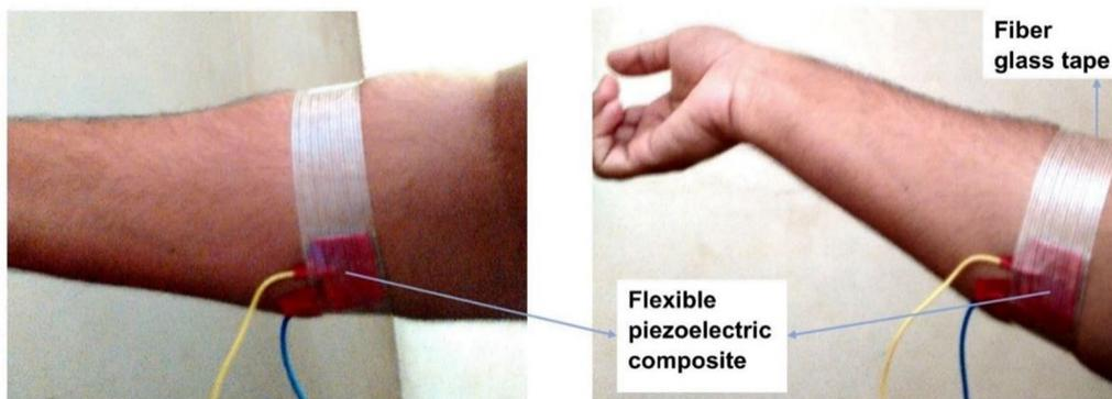
**Figure 2.** Flexible piezoelectric composite specimen wrapped around the flexor carpi muscle for muscle activity measurement.
