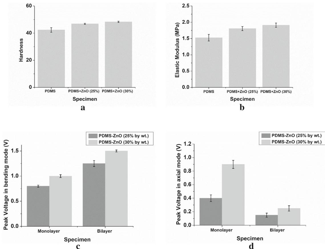
**Figure 3.** (a) Hardness of pure PDMS and PDMS–ZnO composites measured using Shore-A hardness tester. (b) Elastic modulus of pure PDMS and PDMS–ZnO composites calculated from the hardness values. (c) Peak voltage generated from the piezoelectric composite specimen in the bending mode of operation. (d) Peak voltage generated from the piezoelectric composite specimen in the axial mode of operation.
