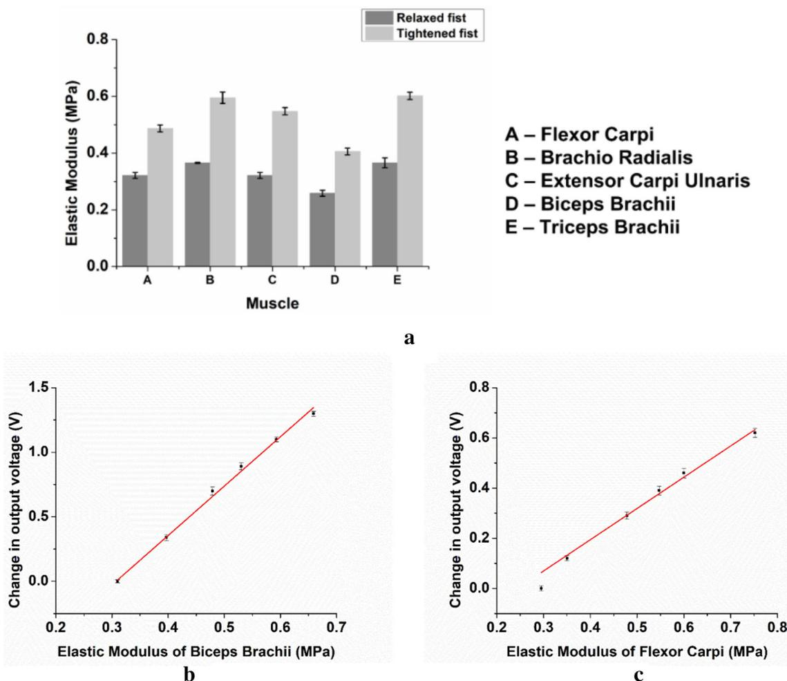
**Figure 4.** (a) Change in elastic modulus of different muscles with the tightening and relaxing of the fist. (b) Change in the output voltage of sensor vs. elastic modulus of biceps brachii muscle. (c) Change in the output voltage of sensor vs. elastic modulus of flexor carpi muscle.
