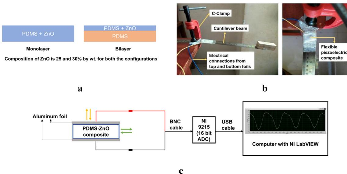
**Figure 1.** (a) Schematic of the monolayer and bilayer configurations of the fabricated composites. (b) Side and top views of the setup for testing the piezoelectric properties of the composite in bending mode of operation. (c) Schematic of the measurement setup. Green arrows indicate the direction of applied force in bending mode and yellow arrows indicate the direction of applied force in the axial mode of operation.
