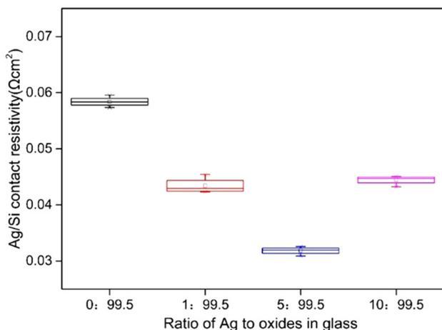
**Figure 5.** Resistivity of the Ag/Si contact with different ratios of Ag to oxides in glass.
