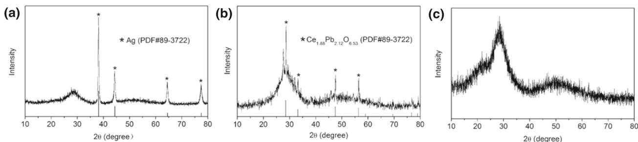
**Figure 1.** XRD patterns of products from glass preparation using different raw materials: (a) Ag powder and oxides not including  $\text{CeO}_2$ ; (b) Ag powder and oxides including  $\text{CeO}_2$  and (c) oxides including  $\text{CeO}_2$ .
