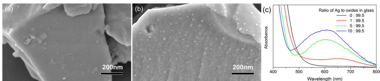
**Figure 4.** SEM images of glass powder (a) containing Ag and (b) not containing Ag. (c) UV–visible spectra of glasses containing different contents of Ag.
