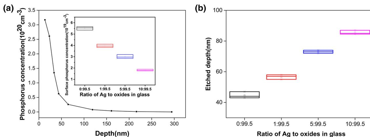
**Figure 7.** (a) Phosphorus concentration distribution curve of a raw Si wafer before Ag paste metallization on it. The inset in (a) shows the surface phosphorus concentrations of Si wafers after Ag paste metallization using glass with different ratios of Ag to oxides. (b) Etched depths of Si wafers by Ag paste metallization, which were estimated according to the surface phosphorus concentrations.
