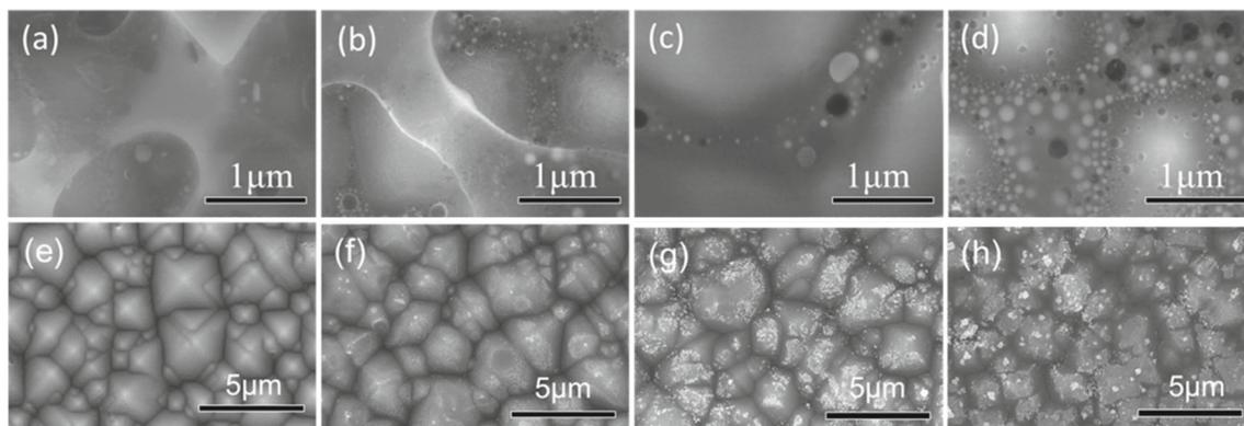
**Figure 6.** SEM images of sintered Ag/Si contact interface. (a–d) The surface where the Ag electrodes were removed and the interface glass layer was exposed. (e–h) The surface where both the Ag electrodes and glass layer were removed. Here the ratios of Ag to oxides in glass are (a, e) 0:99.5, (b, f) 1:99.5, (c, g) 5:99.5 and (d, h) 10:99.5, respectively.
