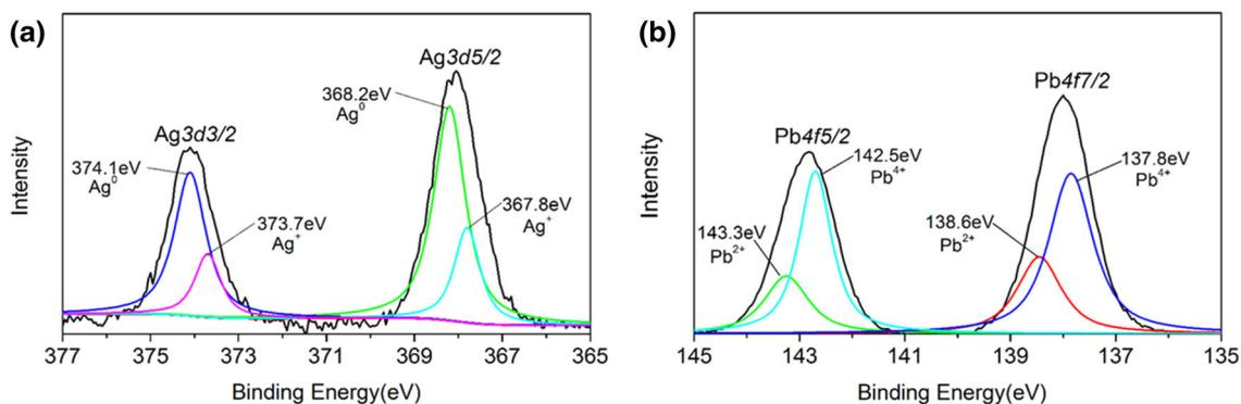
**Figure 3.** XPS spectra of (a) Ag and (b) lead elements in the glass.
