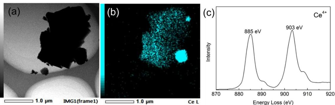
**Figure 2.** TEM analysis of Ce-containing glass: (a) TEM image of glass particles, (b) EDS elemental mapping to show Ce element distribution in glass and (c) EELS of Ce element.
