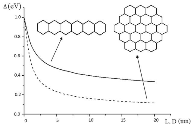
**Figure 2.** Dependence of the effective width of the PL spectrum  $\Delta$  on the size of the quantum dot  $L, D$ . The solid curve is  $\Delta_L$  and the dotted curve is  $\Delta_D$ . Two types of dimers:  $\Delta_L$  is the linear sandwich cluster of benzene rings of length  $L$ ; and  $\Delta_D$  is the cluster of sandwich benzene rings in the form of a disk with a diameter  $D$ . Cross size  $d_{C6}$  of the benzene ring is 0.28 nm.
