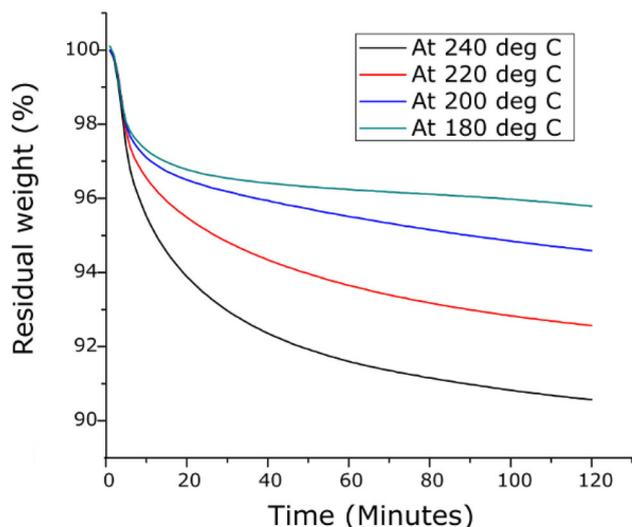
Figure 5. Isothermal TGA of KE-300 at various temperatures.
