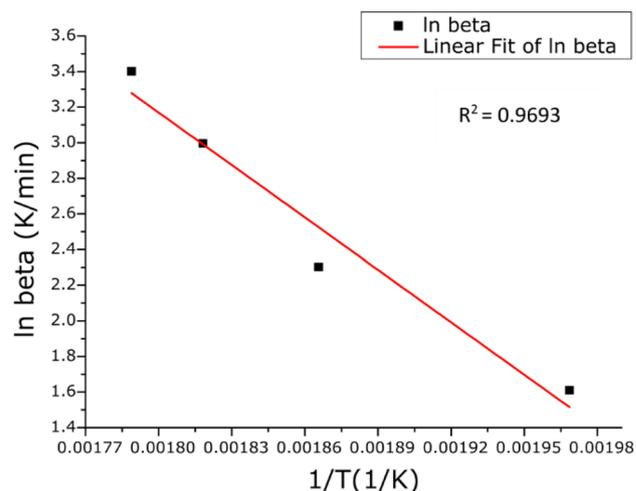
**Figure 4.** FWO plot for 5% of conversion of KE-300.
