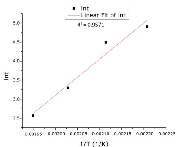
Figure 6. Life time vs. temperature plot for 5% of conversion of KE-300.
