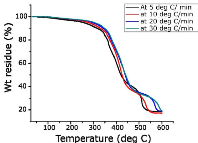
**Figure 3.** Non-isothermal degradation at different heating rates.
