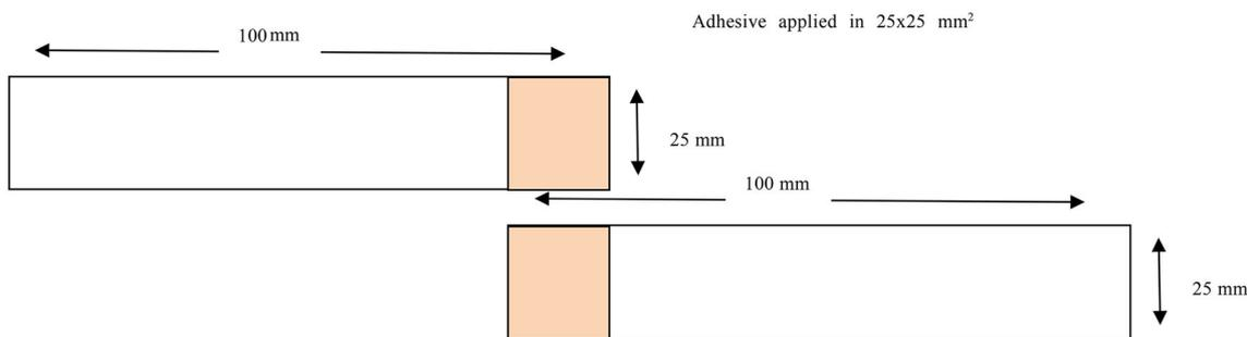
Figure 1. Diagram showing plates with adhesive.
