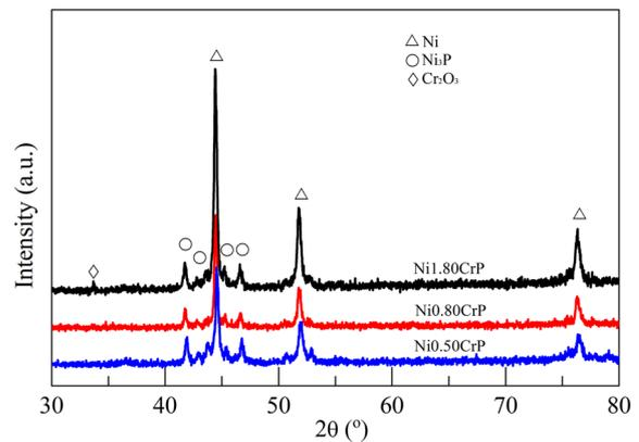
**Figure 7.** XRD patterns of NiCrP alloy coatings with different Cr contents after being oxidized at 400°C for 10 h.
