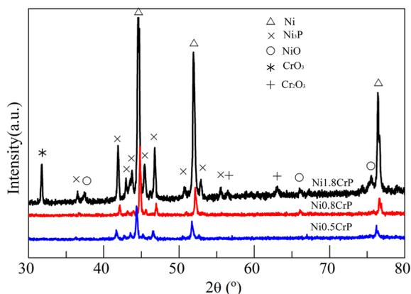
**Figure 8.** XRD patterns of NiCrP alloy coatings with different Cr contents after being oxidized at 500°C for 10 h.
