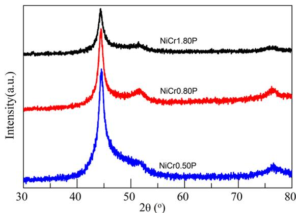
**Figure 6.** XRD patterns of NiCrP alloy coatings with different Cr contents after being oxidized at 300°C for 10 h.
