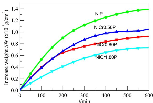
**Figure 3.** Isothermal oxidation curves of NiP and NiCrP alloy coatings at 500°C.
