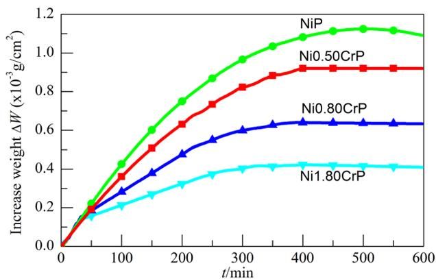
**Figure 2.** Isothermal oxidation curves of NiP and NiCrP alloy coatings at 400°C.
