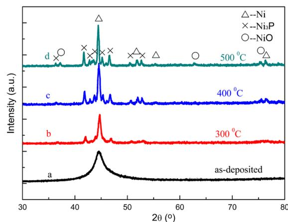
**Figure 4.** XRD patterns of (a) the as-deposited NiP coating, and isochronally heated to the completion temperature of (b) 300, (c) 400 and (d) 500°C, respectively.
