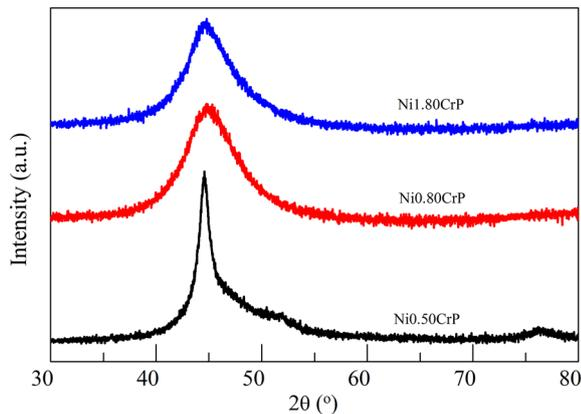
**Figure 5.** XRD patterns of NiCrP alloy coatings with different Cr contents.
