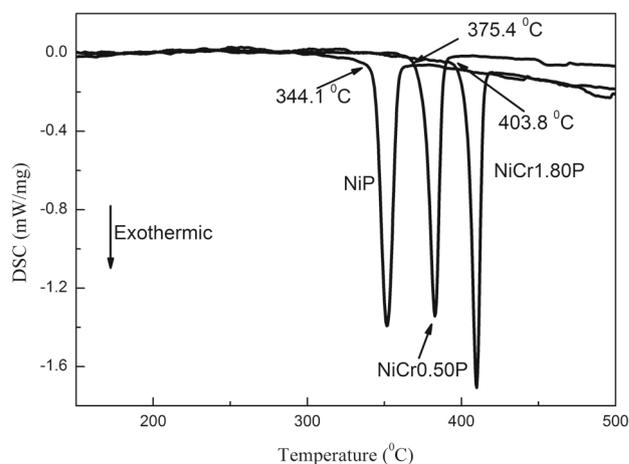
**Figure 1.** DSC curves of NiP and NiCrP amorphous alloy coatings.
