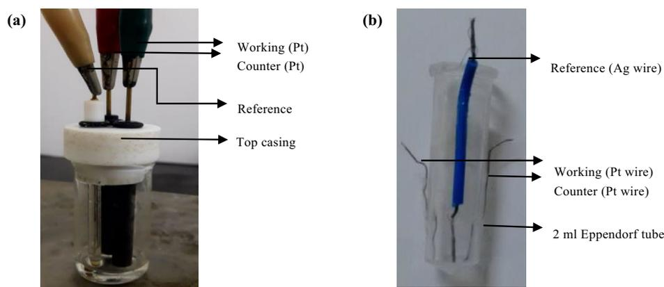
**Figure 1.** (a) Standard electrochemical cell with a platinum working and a counter electrode and Ag/AgCl as the reference electrode assembled in a top casing for measuring 1 ml of enzymatic reaction in a 10 ml of glass vessel. (b) Fabricated mini electrochemical cell in an Eppendorf tube of 2 ml volume to measure enzymatic reactions of 0.2 ml. Two Pt wires, as shown, served as the working and the counter electrodes and a silver wire (with sleeve) as the reference electrode.
