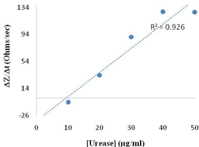
**Figure 4.** Impedance–time measurement as a function of urease concentration from 0 to  $50 \mu\text{g ml}^{-1}$  measured at 100 kHz. The experiment was performed in 3 mM urea contained in 5 mM Tris-HCl, pH 7.2 in an assay volume of 1 ml using the standard three-electrode system.
