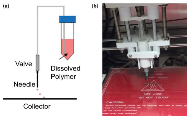
**Figure 1.** Process of solvent-cast 3D printing: (a) process diagram and (b) example of the operation of the printer to make polymer film (source: authors).
