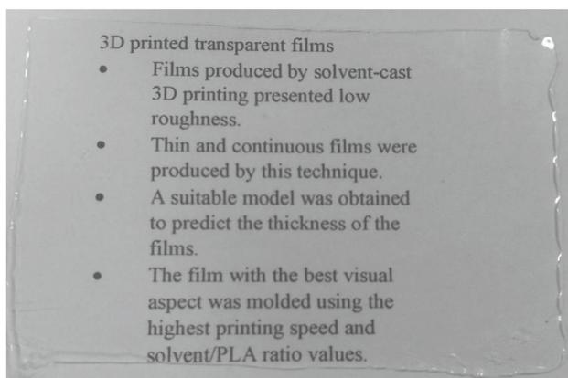
**Figure 5.** 3D printed film of the 60/15:1 sample.
