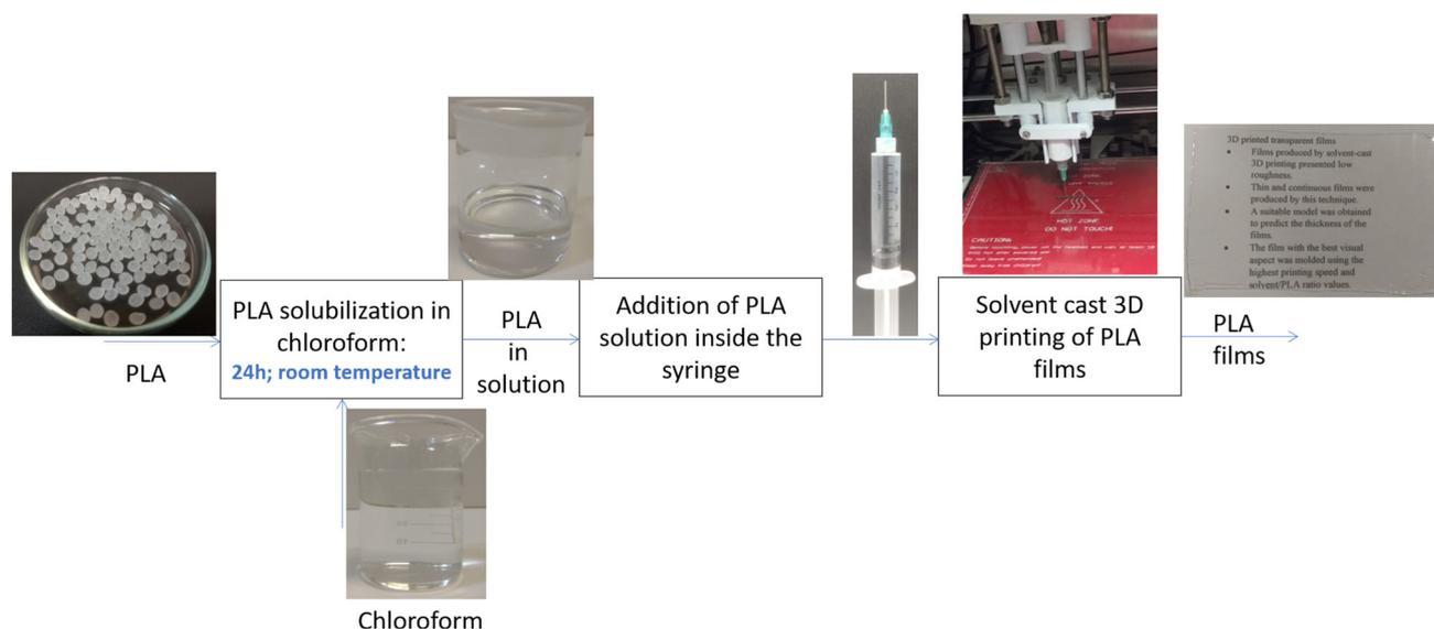
**Figure 2.** Solvent-cast 3D printing method by liquid deposition modelling.
