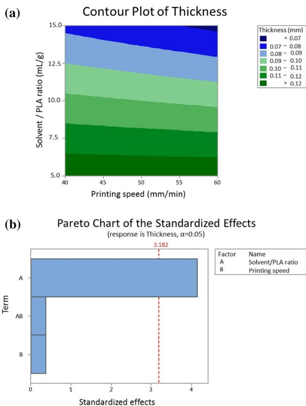
**Figure 3.** (a) Contour plot and (b) Pareto chart of thickness with 95% confidence.
