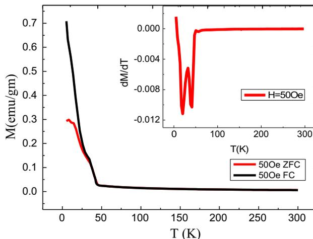
**Figure 4.** Temperature-dependence magnetization was measured under  $H$  is with FC and ZFC modes. Inset  $dM/dT$  vs.  $T$  curves in ZFC mode for  $H = 50$  Oe.
