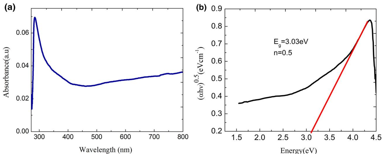
**Figure 2.** (a) Room temperature optical absorption spectrum of GLMO. (b) Graph of  $(\alpha h\nu)^{0.5}$  vs. energy  $(h\nu)$  of the incident photon.
