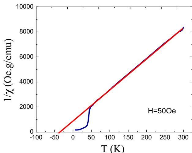
**Figure 5.** Inverse susceptibility vs. temperature graph is plotted in ZFC mode for the field values  $H = 50$  Oe.
