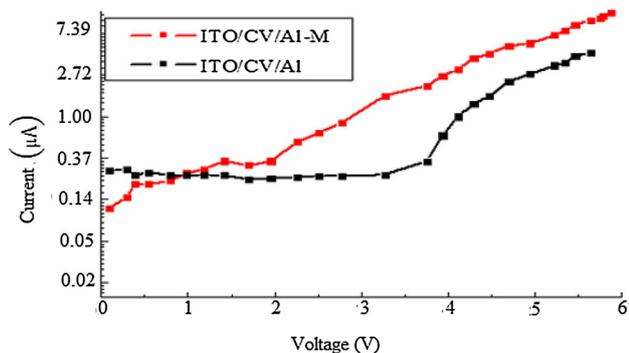
**Figure 4.** Semi-logarithmic plot of ITO/CV/Al-based organic device and ITO/CV/Al-M-based organic device.
