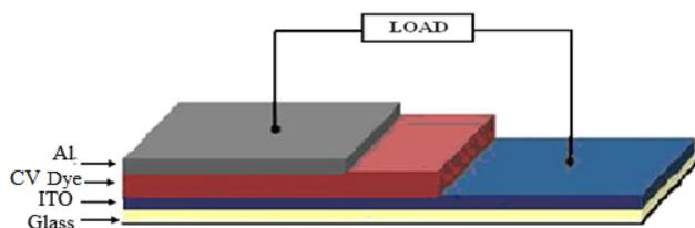
**Figure 2.** Schematic diagram of a sandwich-type organic device, in which CV dye is sandwiched inbetween the two electrodes.
