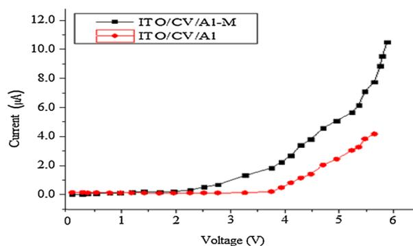
**Figure 3.** Dark  $I\text{--}V$  characteristic of ITO/CV/Al-based organic device and ITO/CV/Al–M-based organic device.
