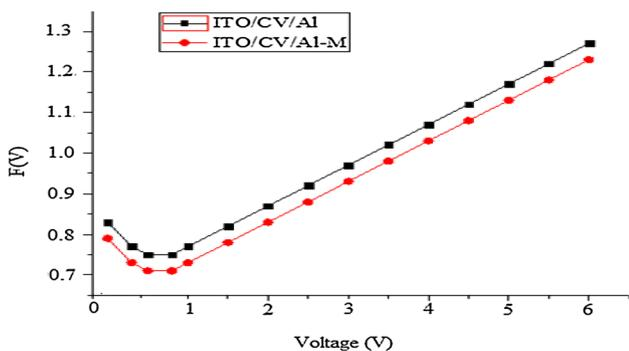
**Figure 5.** Norde function  $F(V)$ - $V$  plot of ITO/CV/Al structure and ITO/CV/Al-M structure.
