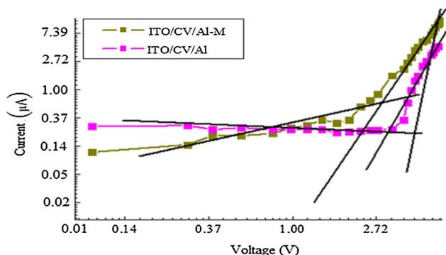
**Figure 6.**  $\ln I$ - $\ln V$  plot of ITO/CV/Al structure and ITO/CV/Al-M structure.
