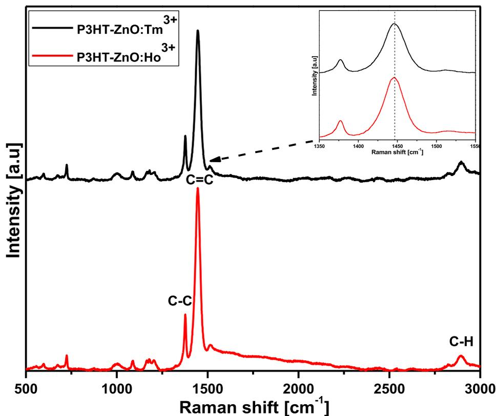
**Figure 3.** Raman spectra of P3HT-ZnO:Ho<sup>3+</sup> and P3HT-ZnO:Tm<sup>3+</sup> film.
