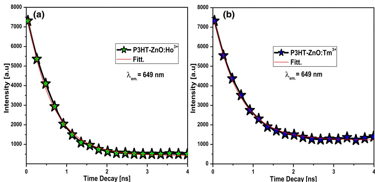
**Figure 4.** Time-resolved fluorescence decays of P3HT-ZnO:Ho<sup>3+</sup> and P3HT-ZnO:Tm<sup>3+</sup> films.
