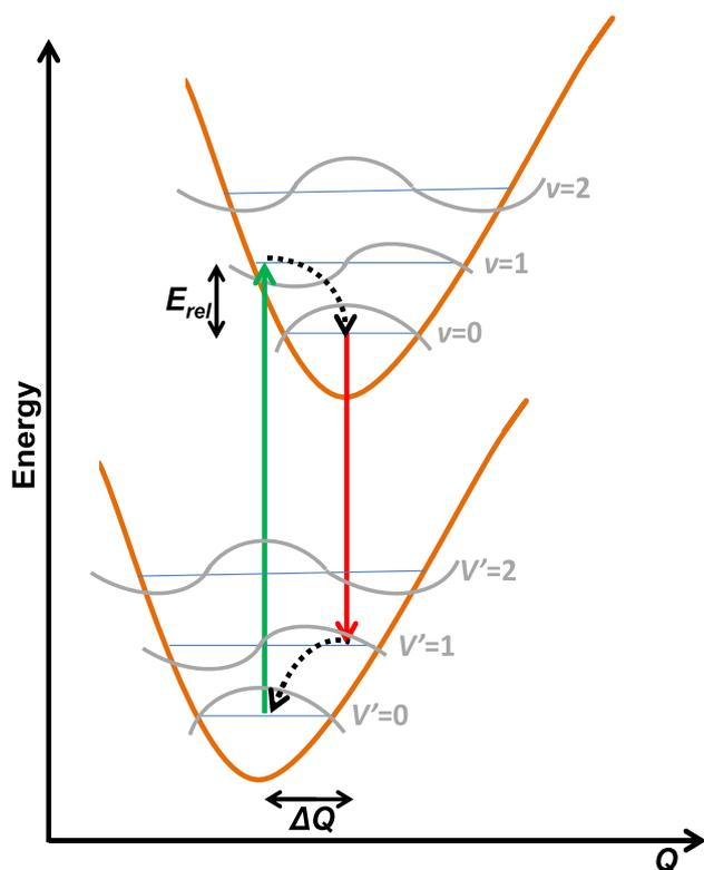
**Figure 1.** Schematic drawing of a vibronic transition in P3HT.  $E_{rel}$  denotes the relaxation energy associated with 0–1 electronic transition and  $Q$  represents the nuclear coordinates. Absorption associated with the transition is shown in green and fluorescence emission in red [7].
