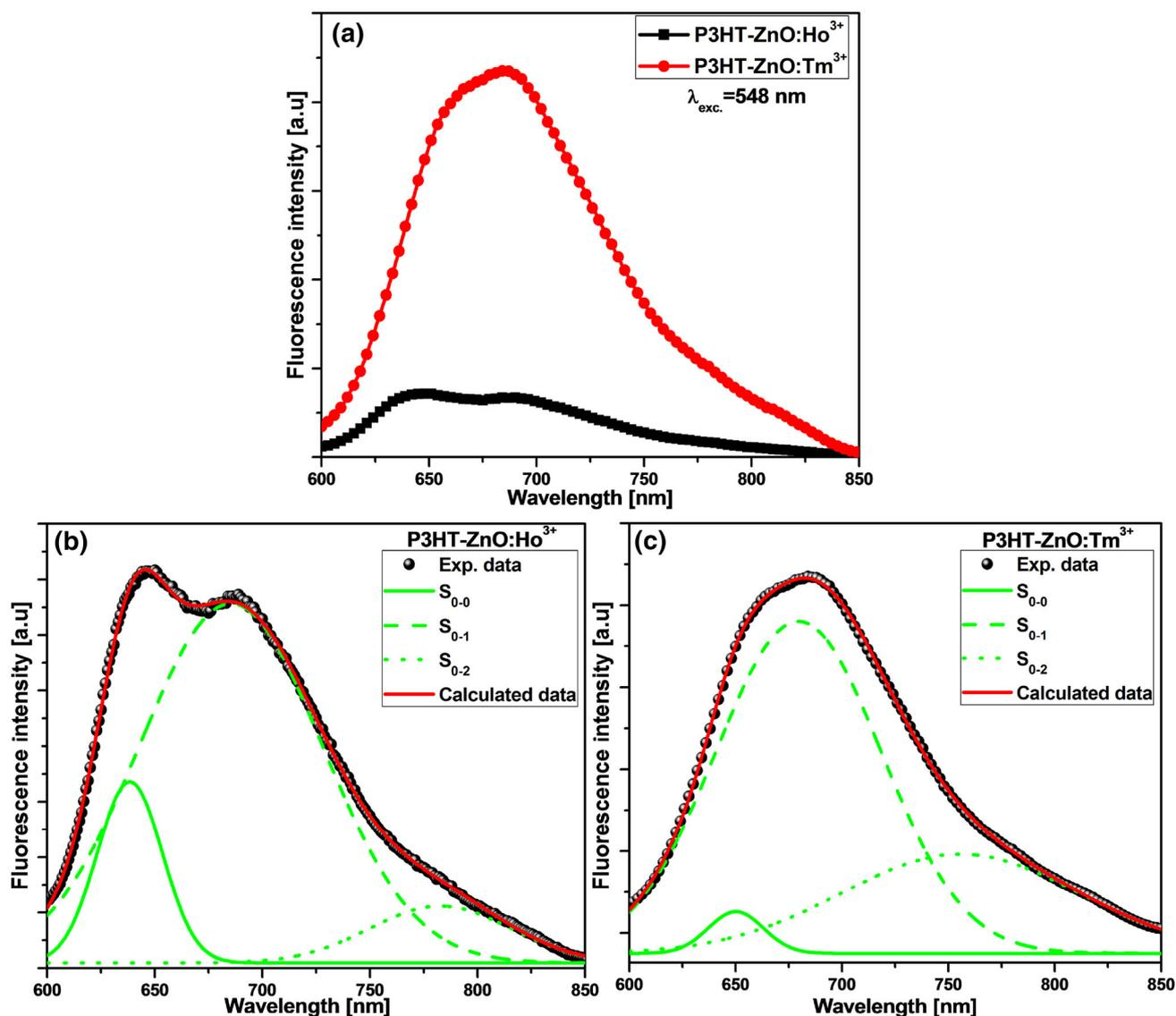
**Figure 2.** (a) Compared fluorescence spectra and (b, c) Gaussian de-convolution of P3HT-ZnO:Ho<sup>3+</sup> and P3HT-ZnO:Tm<sup>3+</sup> films ( $\lambda_{exc} = 548$  nm).
