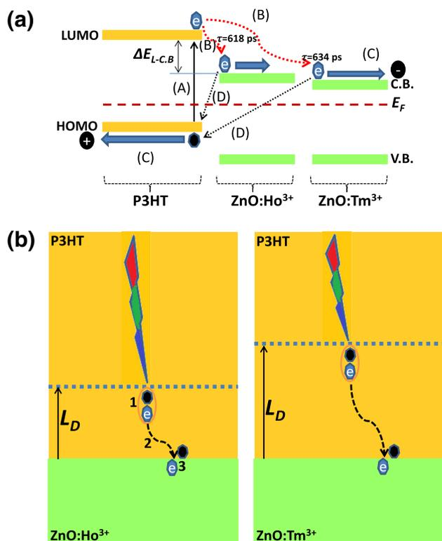
**Figure 5.** (a) Schematic energy diagram and (b) proposed exciton pathway of P3HT-ZnO:Ho<sup>3+</sup> and P3HT-ZnO:Tm<sup>3+</sup> films.
