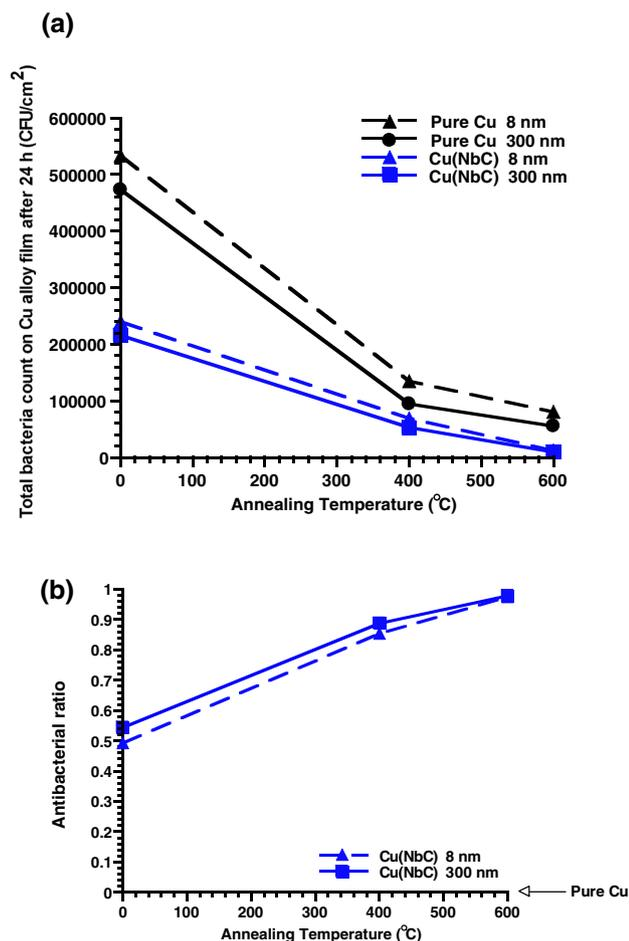
**Figure 4.** Antibacterial efficacy against *S. aureus* BCRC 10451 of the Cu(NbC) alloy and pure-Cu films, of various thicknesses and prior to and after annealing, after 24 h of bacteria exposure—in comparison with that of pure-Cu films, i.e., (a) bacteria count and (b) antibacterial ratio.
