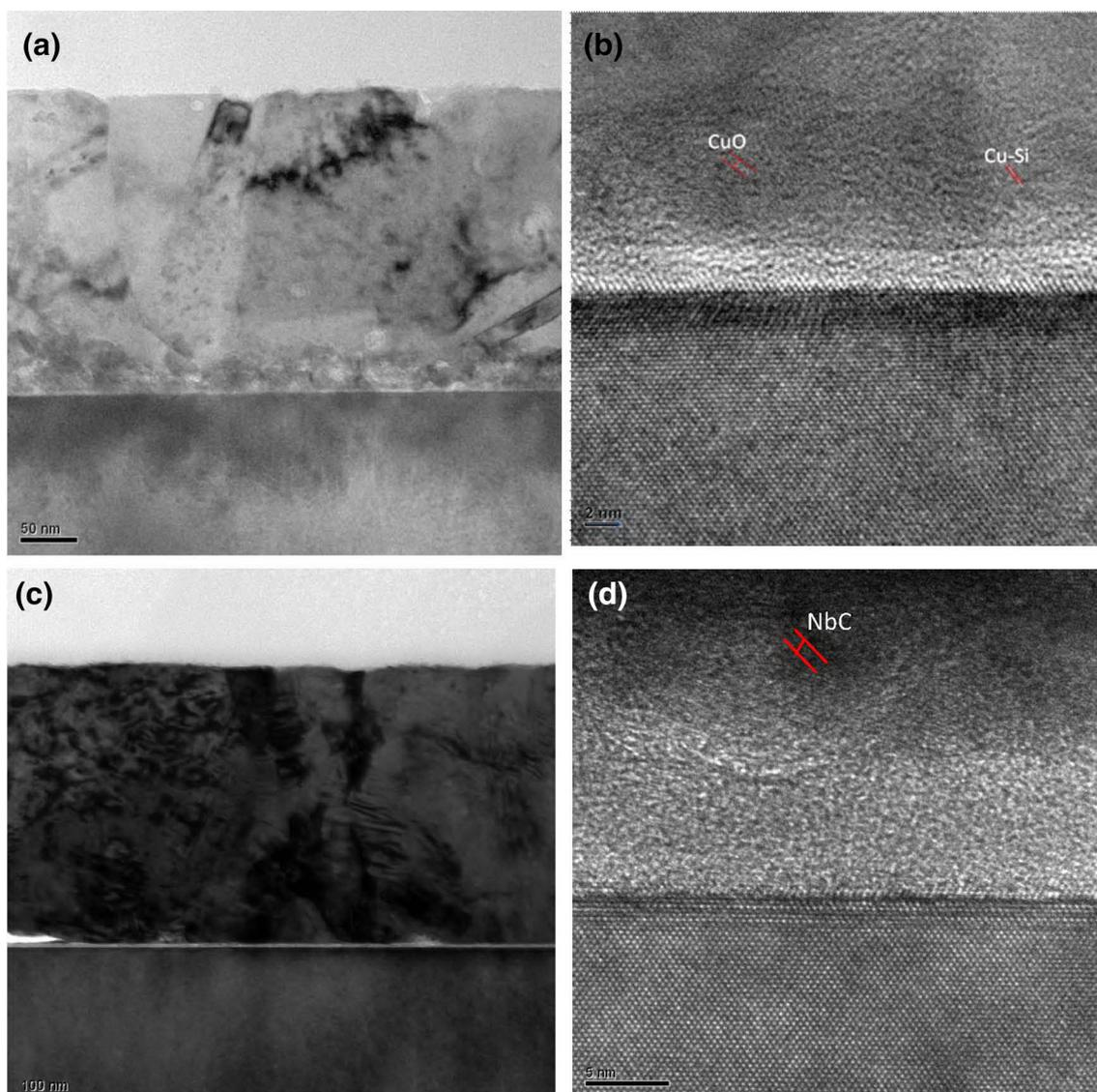
**Figure 3.** Pure Cu (a) TEM and (b) high-resolution TEM images after annealing at 400°C for 1 h; Cu(NbC) alloy (c) TEM and (d) high-resolution TEM images after annealing at 650°C for 1 h (film thickness: 300 nm).
