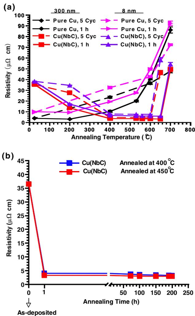
**Figure 2.** (a) Resistivity curves of Cu(NbC) and pure-Cu films, with thicknesses of 8 or 300 nm and sputtered on barrier-free Si substrates, after isothermal and cyclic annealing at various temperatures for various durations as listed inside the figure and (b) the resistivity curves of 300-nm-thick Cu(NbC) films after annealing at 400 or 450°C for 200 h.
