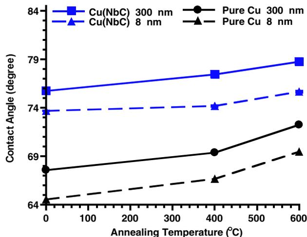
**Figure 5.** Contact-angle variations of Cu(NbC) films in comparison with that of pure-Cu films, before and after annealing.
