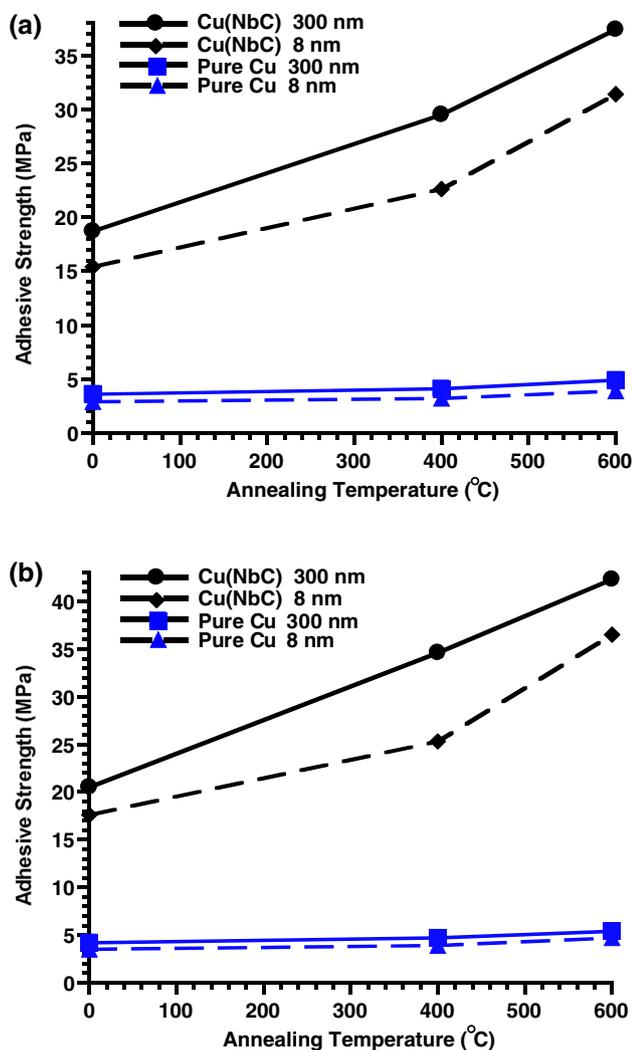
Figure 7. Adhesion test results of pure-Cu and Cu(NbC) films as-deposited and after annealing at 600°C for 1 h for two different film-thicknesses of (a) 8 and (b) 300 nm.
