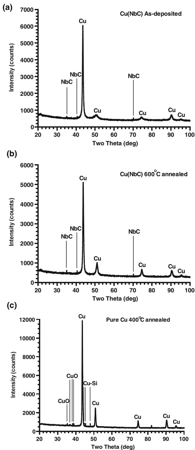
**Figure 1.** (a) XRD pattern of the Cu(NbC) alloy films as-deposited, (b) the XRD pattern of the films after annealing at 600°C for 1 h and (c) for comparison, the XRD pattern of pure-Cu films after annealing at 400°C for 1 h [18].
