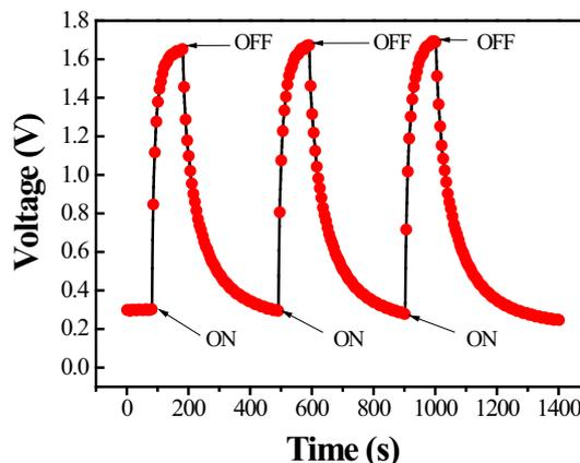
**Figure 2.** Response of ZnO nanoplates film to UV light at  $138^\circ\text{C}$ .
