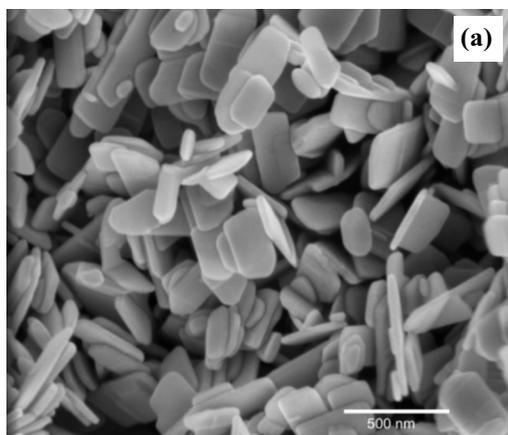
**Figure 1.** (a) SEM image and (b) XRD pattern of ZnO nanoplates.
