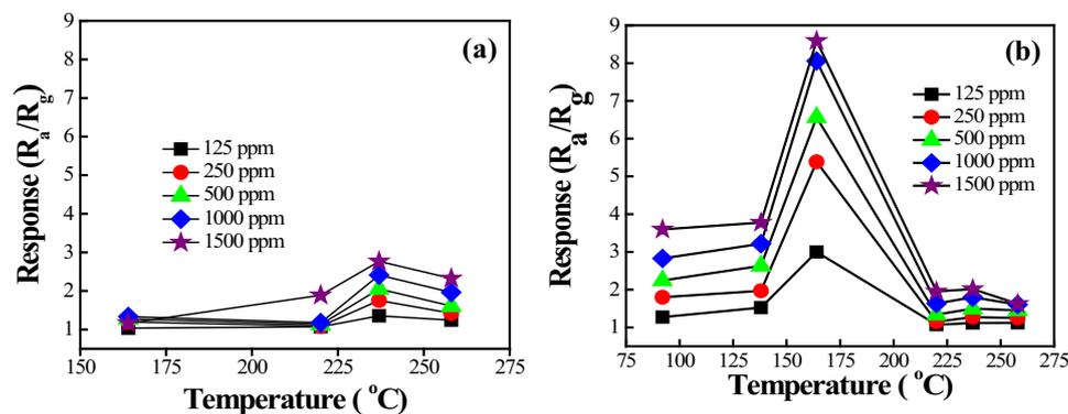
**Figure 5.** Responses of ZnO nanoplate film to ethanol vapour (125–1500 ppm) at various working temperatures in the (a) dark and (b) under UV illumination.
