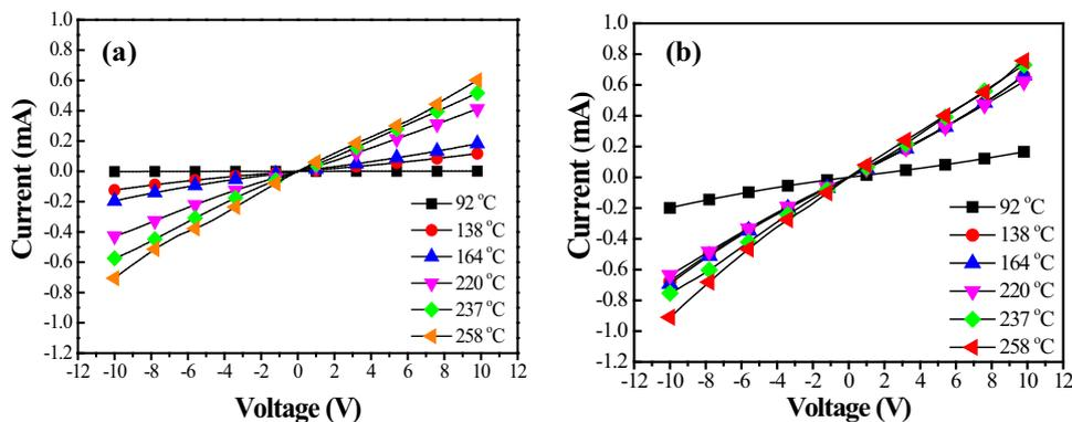
**Figure 3.** *I*–*V* characteristics of ZnO nanoplates film at differential working temperatures in the (a) dark and (b) under UV illumination.
