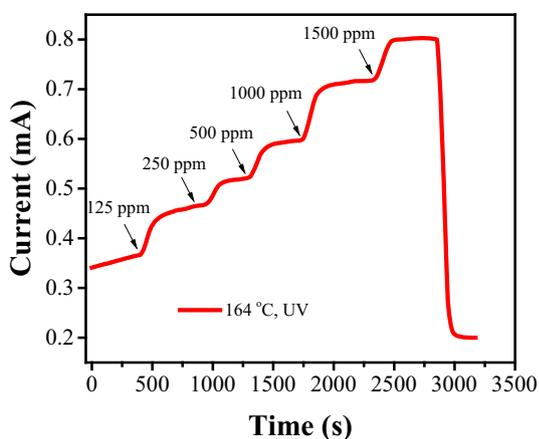
**Figure 4.** Transient response of ZnO nanoplate film to ethanol vapour (125–1500 ppm) under UV illumination at 164 °C.
