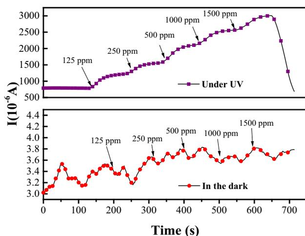
**Figure 6.** Transient response of ZnO nanoplate film to ethanol vapour (125–1500 ppm) at 138°C in the (a) dark and (b) under UV illumination.
