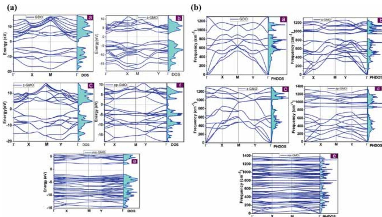
**Figure 5.** (a) Phonon dispersion curves of (a) GDO, (b) a-GMO, (c) z-GMO, (d) ep-GMO and (e) mix-GMO along with the corresponding phonon density of states. (b) Electronic band structures of (a) GDO, (b) a-GMO, (b) z-GMO, (c) ep-GMO and (e) mix-GMO in the Brillouin zone along with electronic density of states [126].
