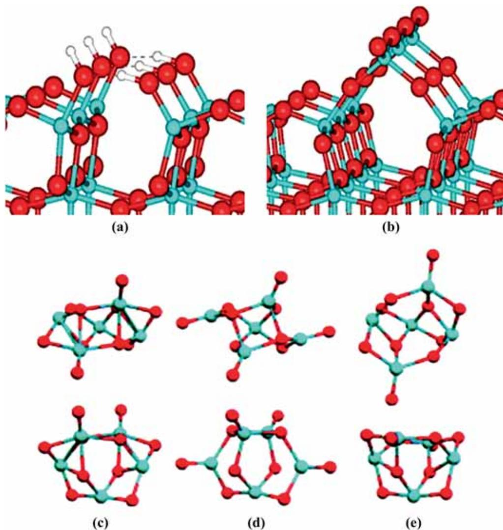
**Figure 4.** Atomic structures covered by (a) (001) surface with 0.5 ml of water [82], and (b) reconstructed clean (001) surface with added molecule [84] with hydrogen, oxygen and titanium represented by white, red and blue dots, respectively. Top and side views of the three  $(\text{TiO}_2)_5$  structures: (c) (PW/VSZ), (d) (B3LYP/VDZ), (e) (B3LYP/LANL2DZ) [93], where oxygen and titanium are represented in red and blue dots, respectively.
