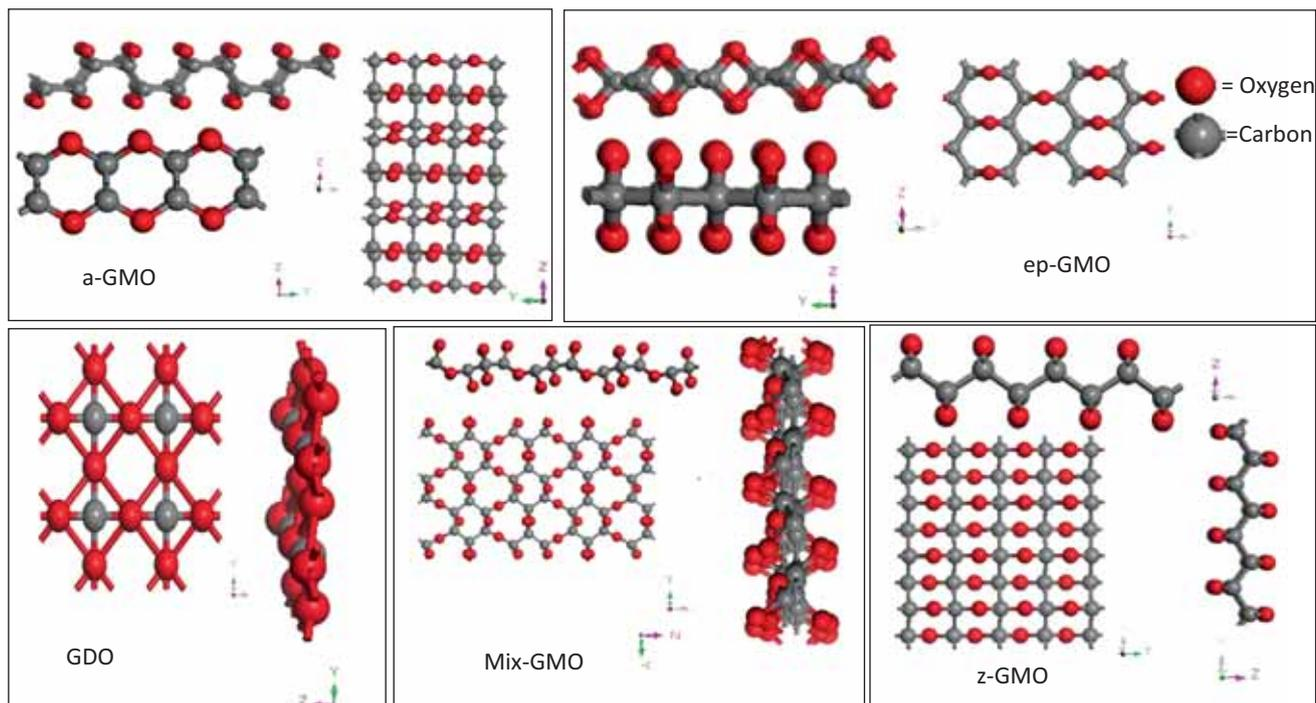
**Figure 6.** Atomic structures of a-GMO, ep-GMO, GDO, mix-GMO and z-GMO, along the  $xy$ ,  $yz$ ,  $xz$  planes. Calculated from lattice parameters [126].
