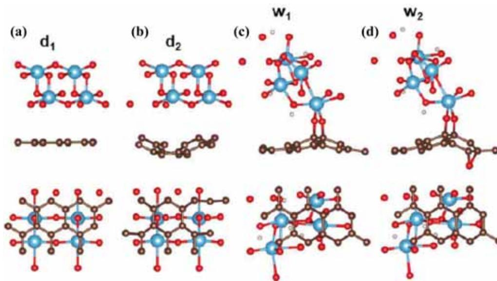
**Figure 7.** Side and top views of graphene–TiO<sub>2</sub> bilayer nanocomposite models with physisorbed (a) *d*<sub>1</sub> and (b) *d*<sub>2</sub> hybrid models and (c) *w*<sub>1</sub> and (d) *w*<sub>2</sub> models [144].
