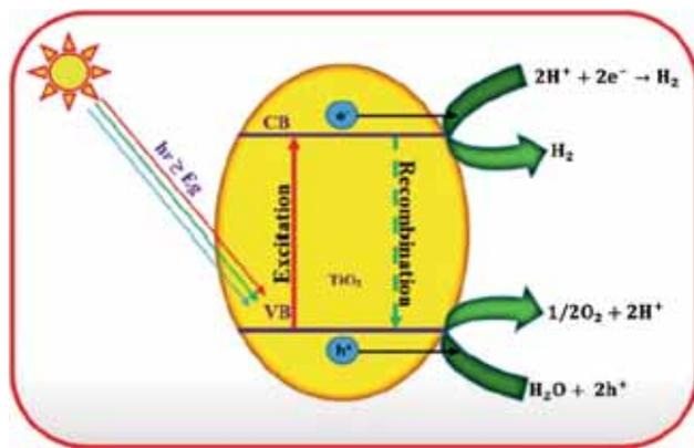
**Figure 1.** The synergistic effect of photocatalytic titania [47].
