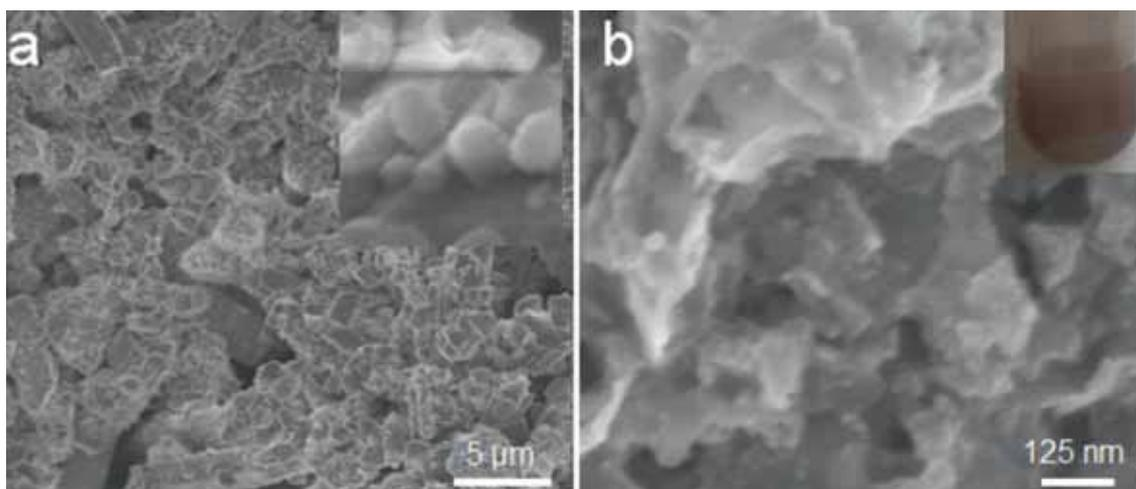
**Figure 6.** SEM images of the as-synthesized Au-MnO<sub>2</sub>-KTiNbO<sub>5</sub> composites after it is used to hydrogenate p-nitrophenol for (a) the first and (b) 21st times, respectively.
