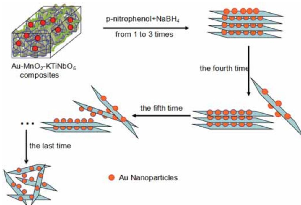
**Scheme 2.** Schematic illustration of the catalytic mechanism of 'layer-by-layer quilt exposure' mode.
