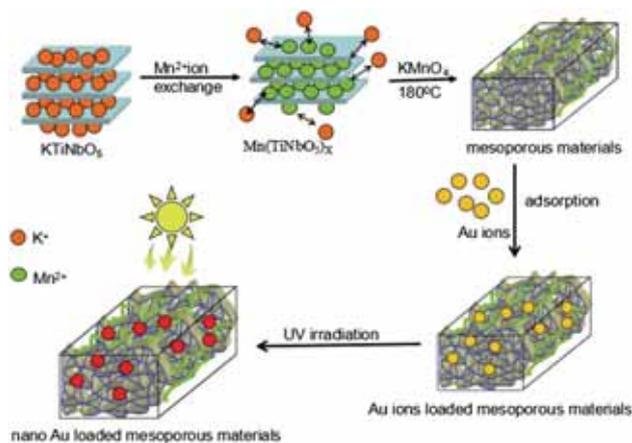
**Scheme 1.** Fabrication of composites of porous KTiNbO<sub>5</sub> loaded with Au nanoparticles.
