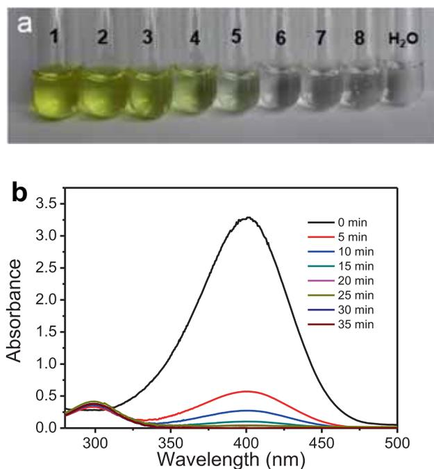
**Figure 4.** (a) The image and (b) UV spectra are showing the hydrogenation effect of Au-MnO<sub>2</sub>-KTiNbO<sub>5</sub> composites on p-nitrophenol (Au-MnO<sub>2</sub>-KTiNbO<sub>5</sub>, 0.25 g; NaBH<sub>4</sub>, 0.528 mol l<sup>-1</sup>, 30 ml and p-nitrophenol, 5 mmol l<sup>-1</sup>, 20 ml).
