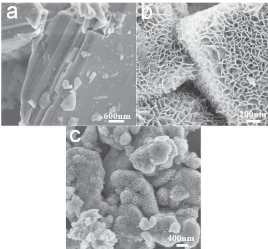
**Figure 1.** SEM images of the (a) as-synthesized KTiNbO<sub>5</sub>, (b) magnetic oxide-pillared KTiNbO<sub>5</sub> and (c) Au-loaded magnetic oxide-pillared KTiNbO<sub>5</sub>.
