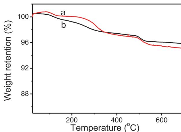
**Figure 2.** TG curves of the as-synthesized porous  $\text{KTiNbO}_5$  (line a) and Au-loaded  $\text{KTiNbO}_5$  composites (line b).
