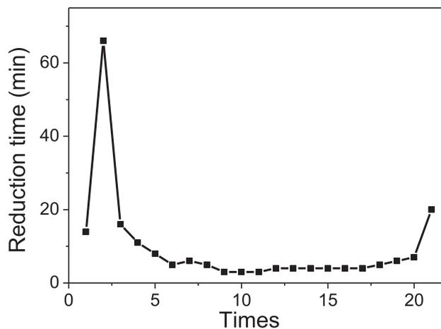
**Figure 5.** Reaction time of the reducing p-nitrophenol with the as-synthesized composites from the first to 21st times.
