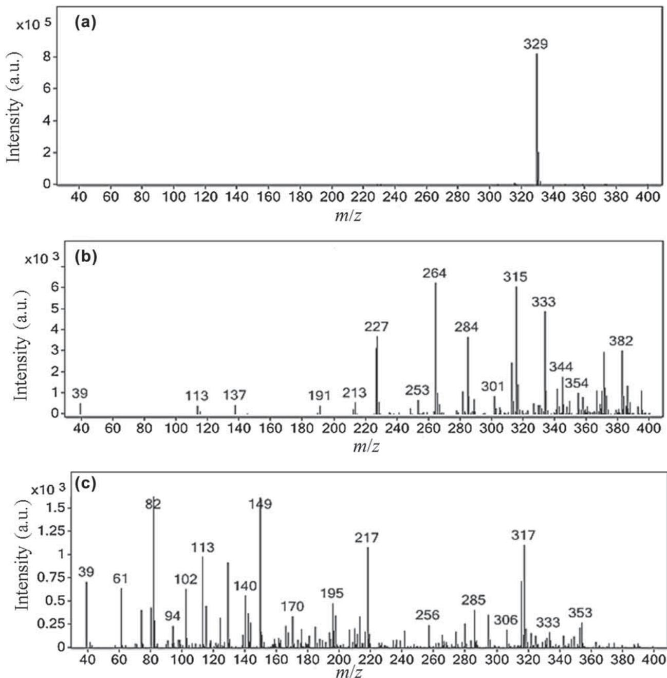
**Figure 10.** Mass spectra of (a) MG dye solution before solar irradiation and (b, c) after solar irradiation in the presence of ZnO NPs for 30 and 90 min, respectively.
