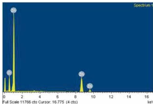
**Figure 2.** EDX spectrum of biosynthesized ZnO NPs.
