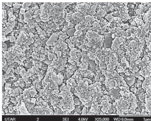
**Figure 3.** FESEM image of green-synthesized ZnO NPs.
