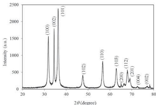
**Figure 1.** XRD pattern of biosynthesized ZnO NPs using *G. mangostana* fruit pericarp extract.
