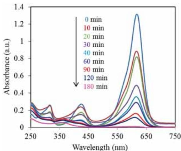
**Figure 7.** Time-dependent UV-Vis absorption spectra of photocatalytic degradation of MG dye in the presence of biosynthesized ZnO NPs.
