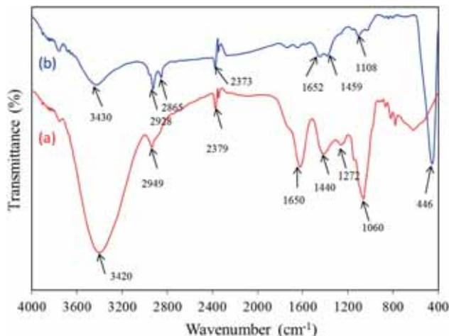
**Figure 6.** FTIR spectra of (a) pure *G. mangostana* fruit pericarp extract and (b) biosynthesized ZnO NPs by using *G. mangostana* fruit pericarp extract.
