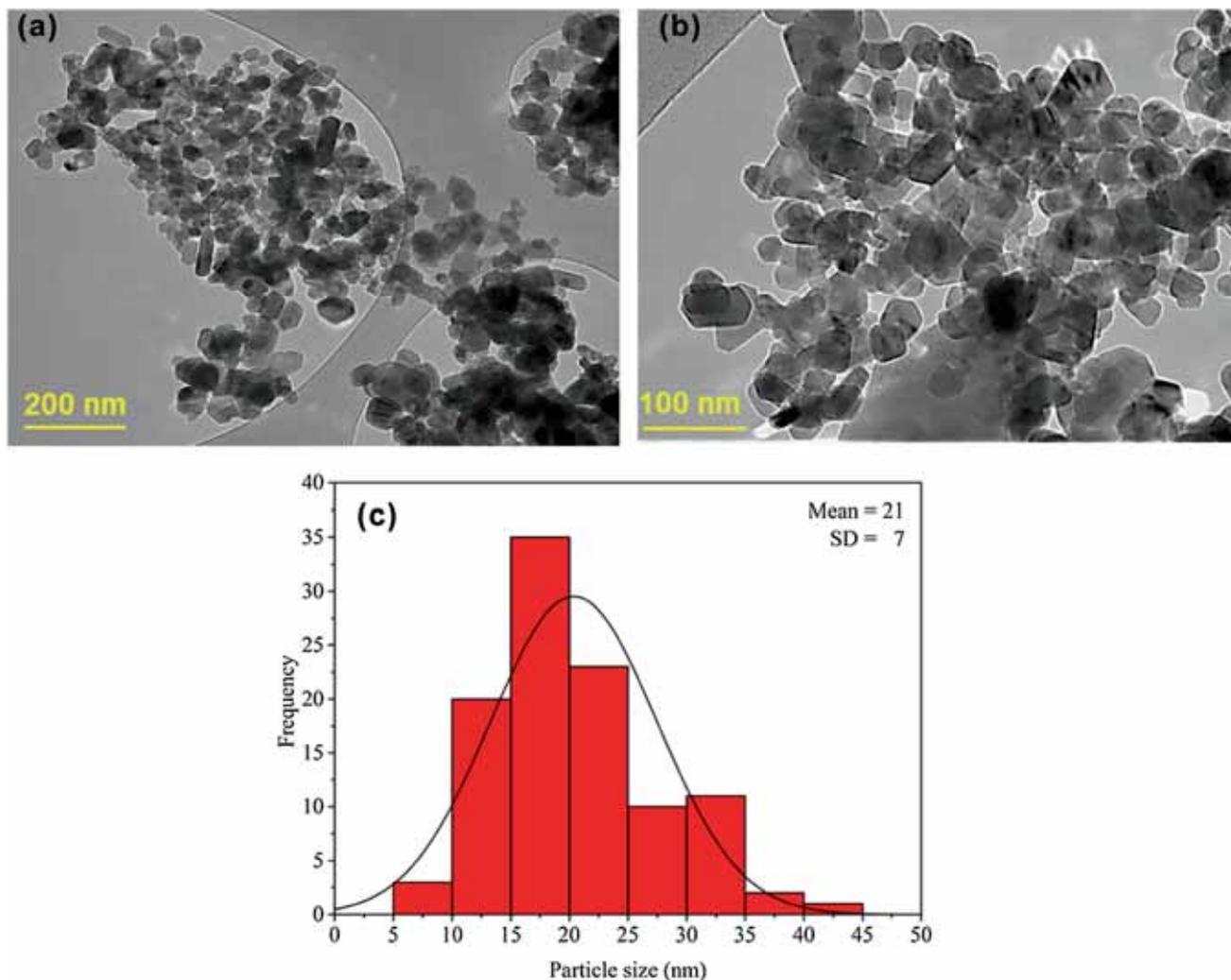
**Figure 4.** TEM images of ZnO NPs forms using *G. mangostana* fruit pericarp extract and histogram of particles size distribution of ZnO NPs.
