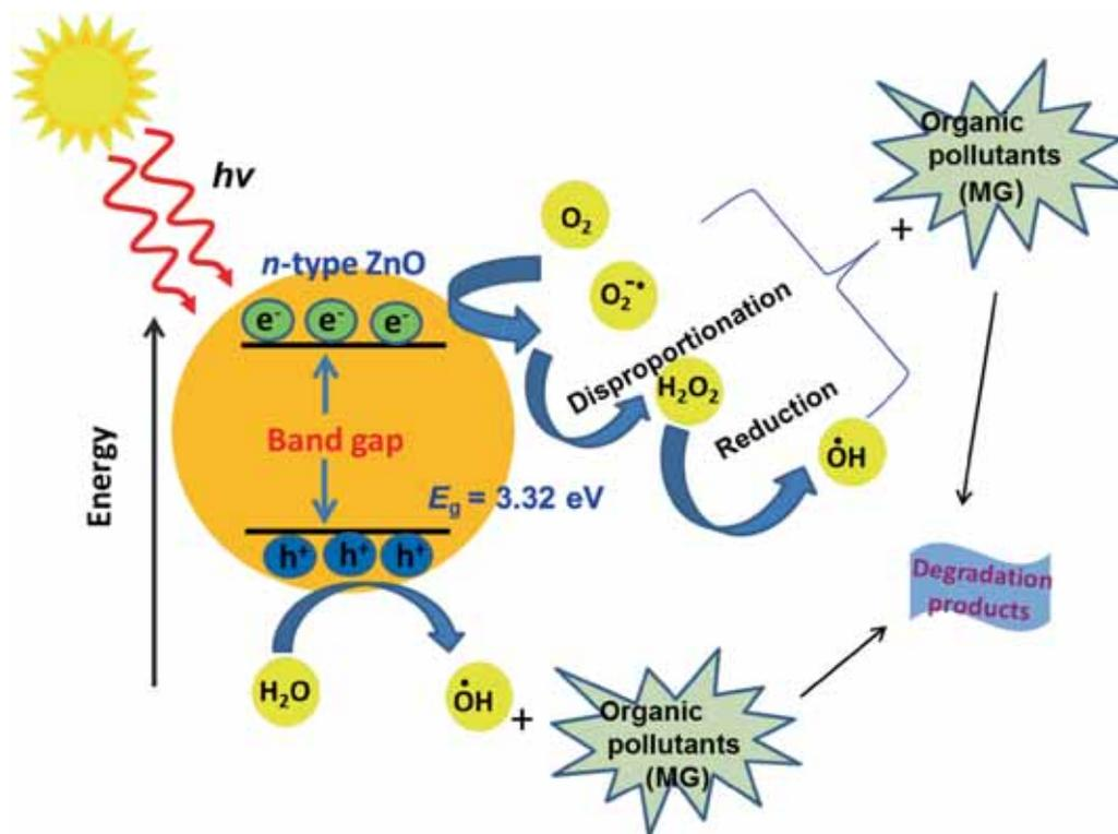
**Scheme 2.** Photocatalytic reaction mechanism of biosynthesized ZnO NPs.
