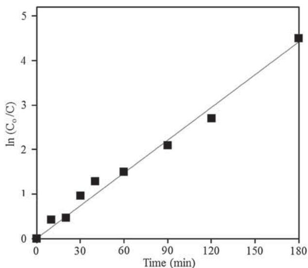
**Figure 12.** Plot of  $\ln(C_0/C)$  vs. time, displaying the photocatalytic degradation of MG dye.
