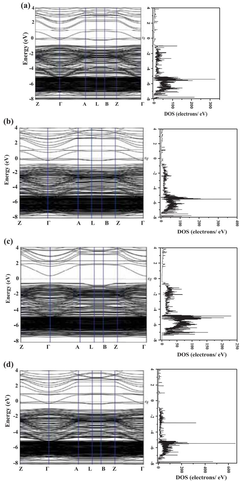
**Figure 3.** Electronic structure of the ZnO NW after adsorption of (a)  $\text{NH}_3$ , (b)  $\text{H}_2\text{O}$ , (c)  $\text{C}_2\text{H}_5\text{OH}$  and (d)  $(\text{CH}_3)_2\text{CO}$  molecules.
