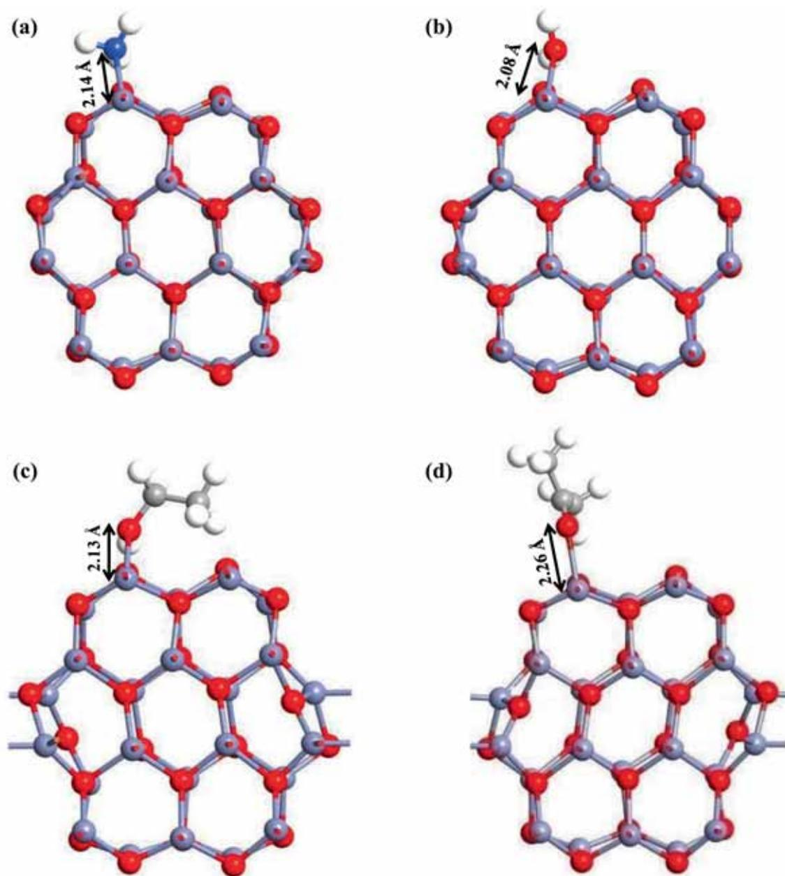
**Figure 2.** Optimized structure of the ZnO NW after the adsorption of (a)  $\text{NH}_3$ , (b)  $\text{H}_2\text{O}$ , (c)  $\text{C}_2\text{H}_5\text{OH}$  and (d)  $(\text{CH}_3)_2\text{CO}$  molecules.
