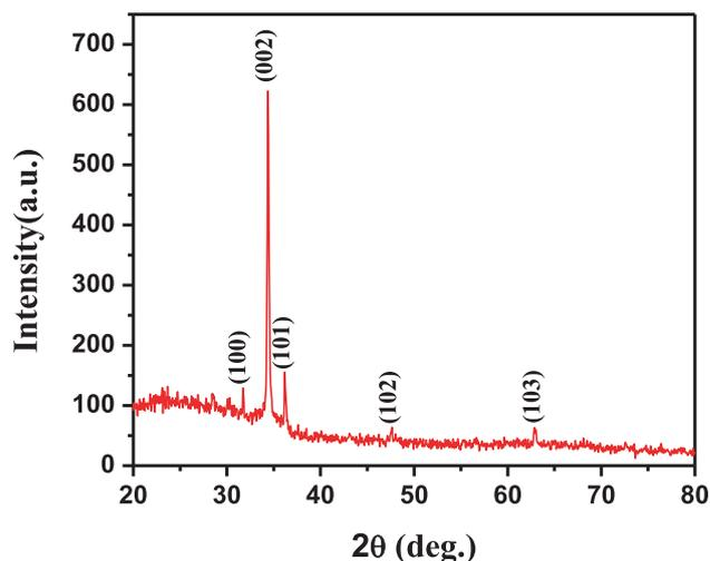
**Figure 5.** XRD pattern of as-deposited ZnO nanowires.
