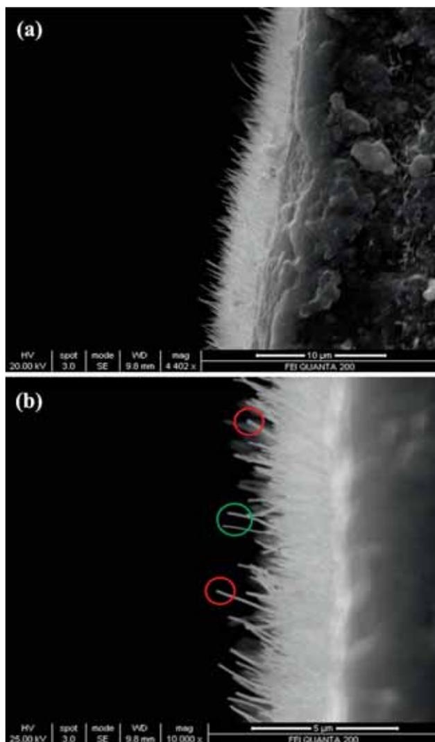
**Figure 4.** Cross-sectional scanning electron micrograph of the SILAR-deposited ZnO at (a) 4402 $\times$  and (b) 10000 $\times$  magnifications.
