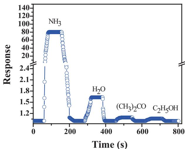
**Figure 6.** Transient response of ZnO NWs towards reducing vapours at 50 ppm.
