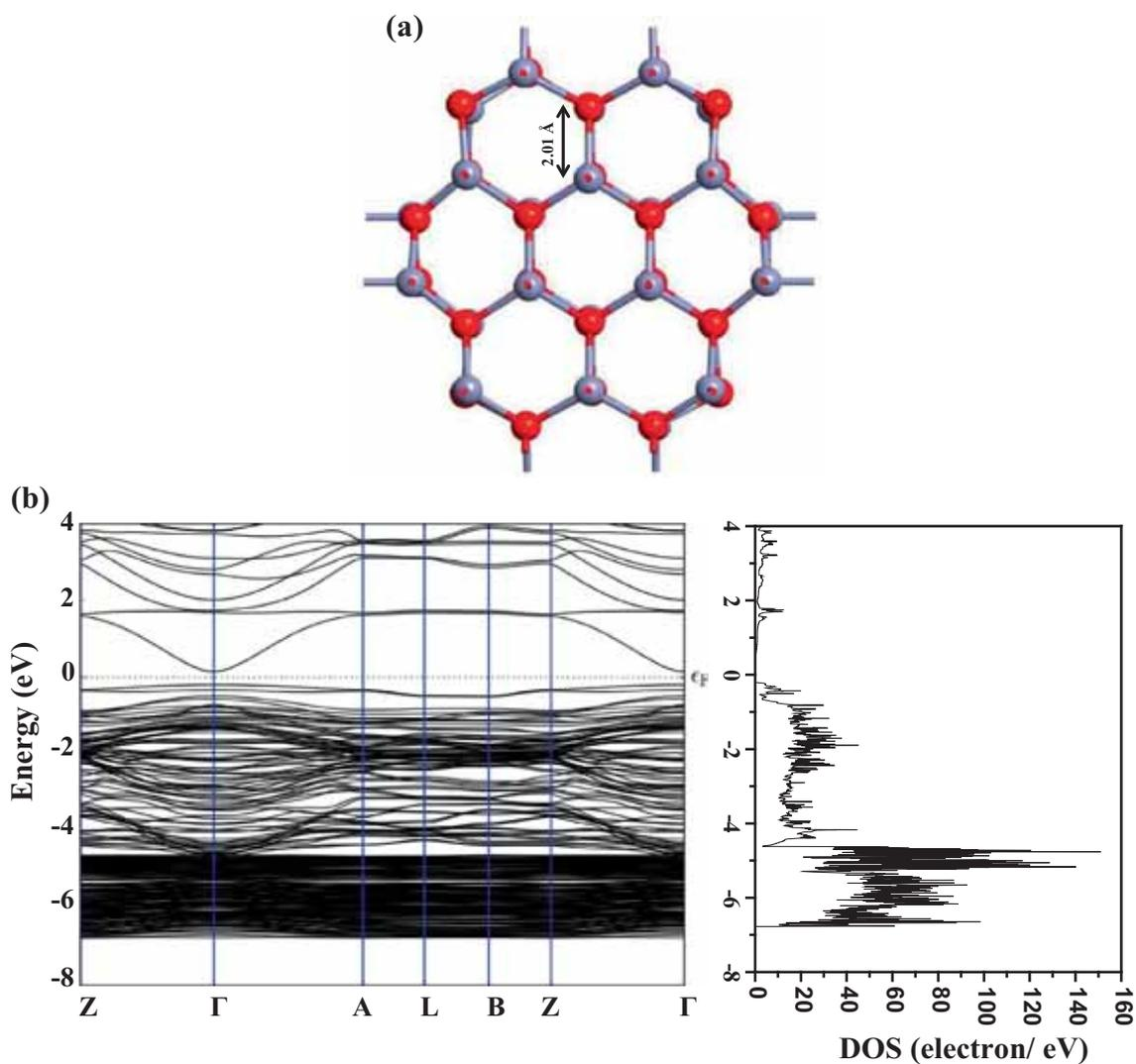
**Figure 1.** (a) Optimized structure of the ZnO nanowire system. (b) Band structure and density of state of the ZnO nanowire.
