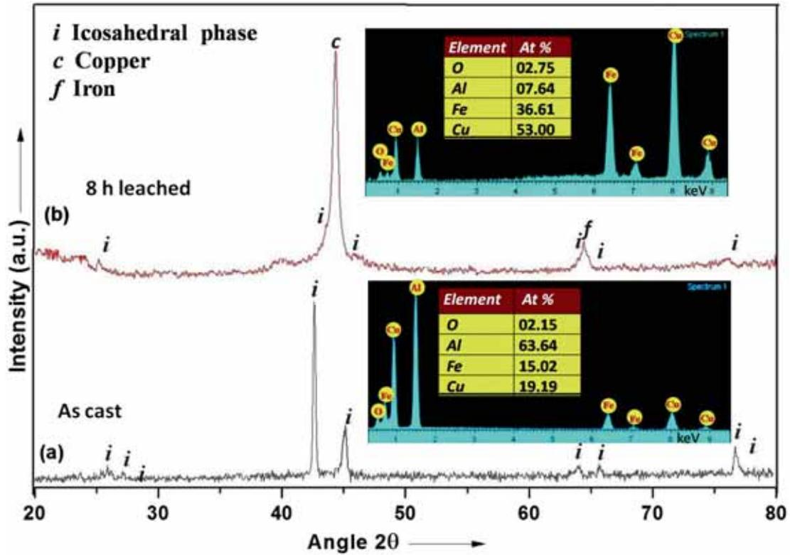
**Figure 1.** X-ray diffraction patterns (a) as-synthesized (i)- $\text{Al}_{65}\text{Cu}_{20}\text{Fe}_{15}$  ribbon and (b) ribbon leached for 8 h with 10 mol of NaOH solution; insets show the corresponding EDX spectra.
