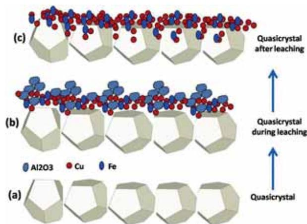
**Figure 5.** A schematic diagram of the leaching process on Al–Cu–Fe QC ribbon surfaces and precipitation of Cu and Fe nanoparticles.
