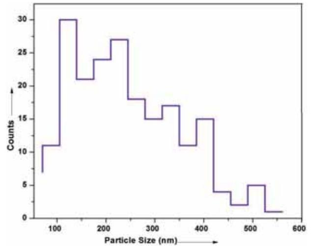
**Figure 3.** Histograms of crystallite size distribution measurements on SEM microstructure of as-synthesized (i)- $\text{Al}_{65}\text{Cu}_{20}\text{Fe}_{15}$  ribbon surface leached for 8 h with 10 mol NaOH solution.
