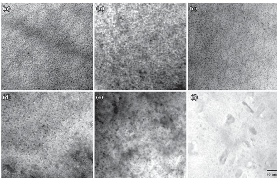
**Figure 1.** TEM micrographs of GISS cast 7075-T6 aged specimens at (a) 120°C for 72 h [4], (b) 120°C for 132 h, (c) 145°C for 6 h, (d) 145°C for 24 h, (e) 145°C for 72 h and of (f) as-received wrought 7075-T651 Al alloy.
