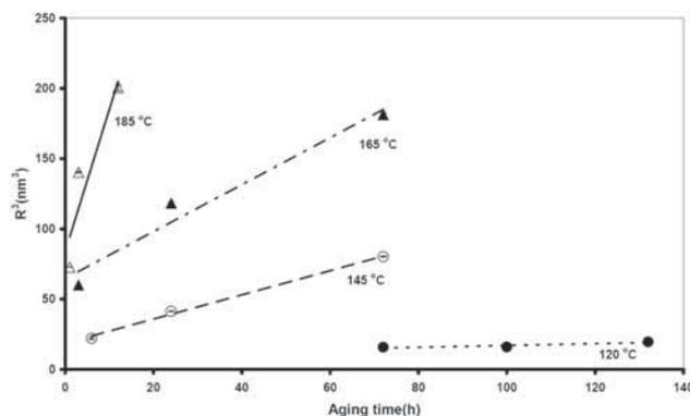
**Figure 6.** Plots of  $R^3$  vs. ageing time for 120, 145, 165 and 185°C show reasonably good fit of linear volume growth models to our data.
