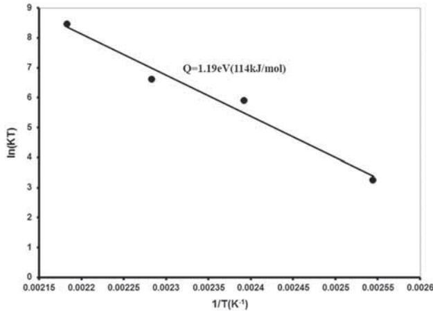
**Figure 7.** A plot  $\ln(KT)$  vs. ageing  $1/T$  is nearly linear displaying a modified Arrhenius type temperature dependency for the coarsening rates.
