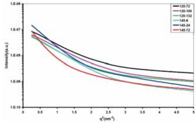
**Figure 2.** Guinier semi-log plots of  $I$  vs.  $q^2$  for the 7075-T6 Al alloy aged at 120°C for 72 h (120–72), 100 h (120–100) and 132 h (120–132); and at 145°C for 6 h (145–6), 24 h (145–24) and 72 h (145–72).
