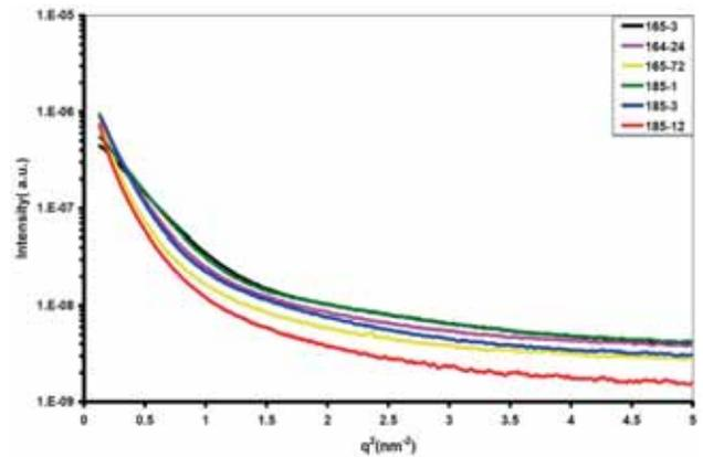
**Figure 3.** Guinier semi-log plots of  $I$  vs.  $q^2$  for the 7075-T6 Al alloy aged at 165°C for 3 h (165–3), 24 h (165–24) and 72 h (165–72); and at 185°C for 1 h (185–1), 3 h (185–3) and 12 h (185–12).
