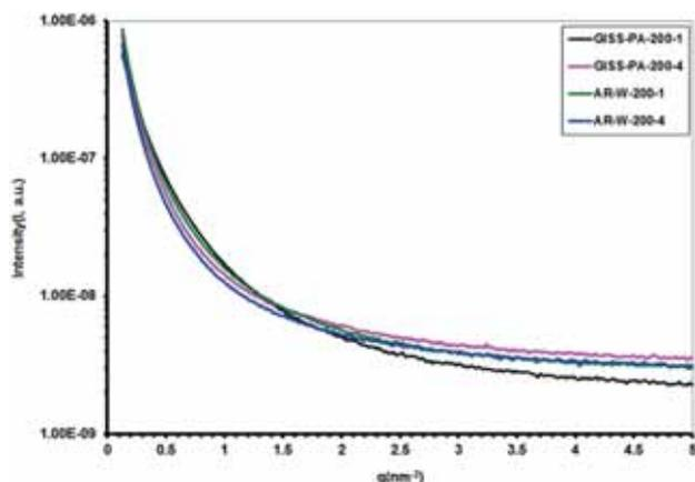
**Figure 5.** Guinier semi-log plots of  $I$  vs.  $q^2$  for the 7075-T6 PA heating at 200°C for 1 h (GISS-PA-200-1) and 4 h (GISS-PA-200-4) and as-received wrought 7075 Al alloy heating at 200°C for 1 h (AR-W-200-1) and 4 h (AR-W-200-4).
