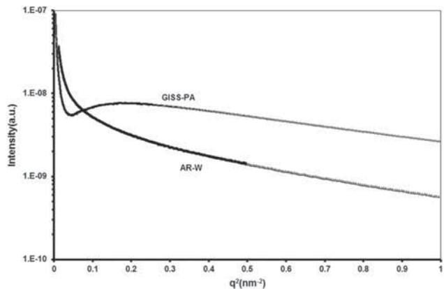
**Figure 4.** Guinier semi-log plots of  $I$  vs.  $q^2$  for the 7075-T6 Al alloy aged at 120°C for 72 h (GISS-PA) and for as-received wrought 7075-T651 Al alloy (AR-W).
