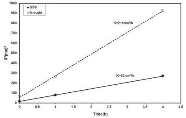
**Figure 8.** Plot  $R^3$  vs. holding time at 200°C for GISS cast 7075-PA (GISS) and wrought 7075 Al alloy (wrought).
