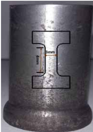
Figure 2. Tensile test dimension on PTCAP processed tube.
